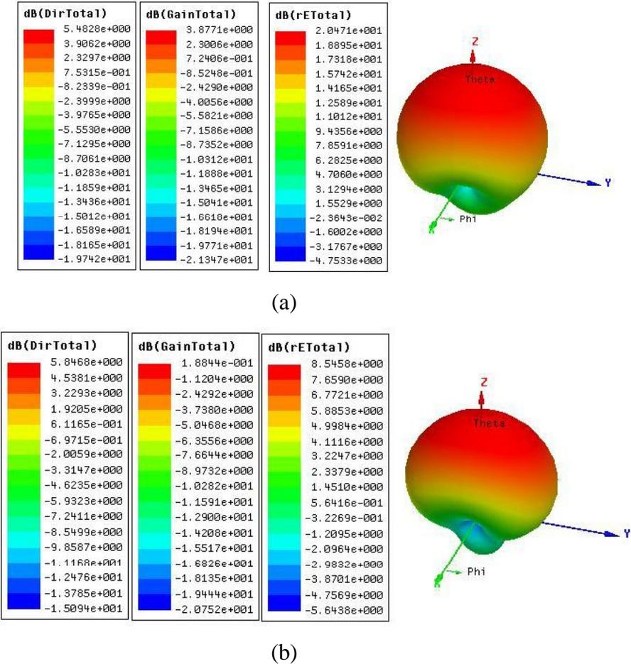
**Figure 4.7 Polar Radiation Characteristics with Directivity, Gain and total E Field (a) PFA at 6.02 GHz (b) TFA at 6.02 GHz**
