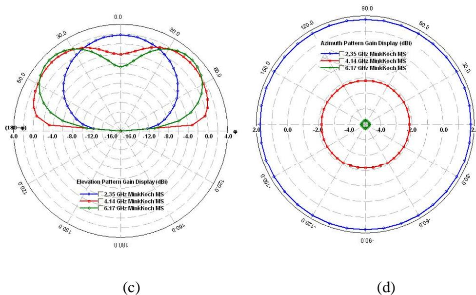
**Figure 4.4 Radiation Patterns (a) Elevation Pattern of Microstrip Fed FA (b) Azimuth Pattern of Microstrip Fed FA (c) Elevation Pattern of CPW Fed FA (d) Azimuth Pattern of CPW Fed FA**
