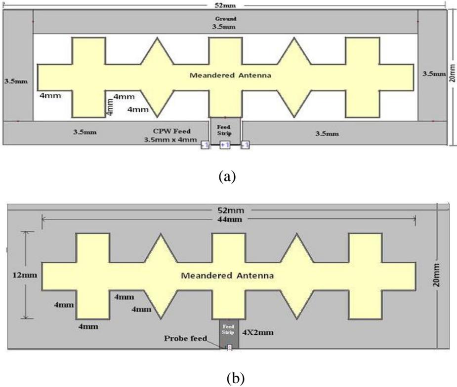
**Figure 4.2 Minkowski-Koch Fractal Patch Antenna CPW Fed Meandered FA (b) Microstrip Fed Meandered FA**
