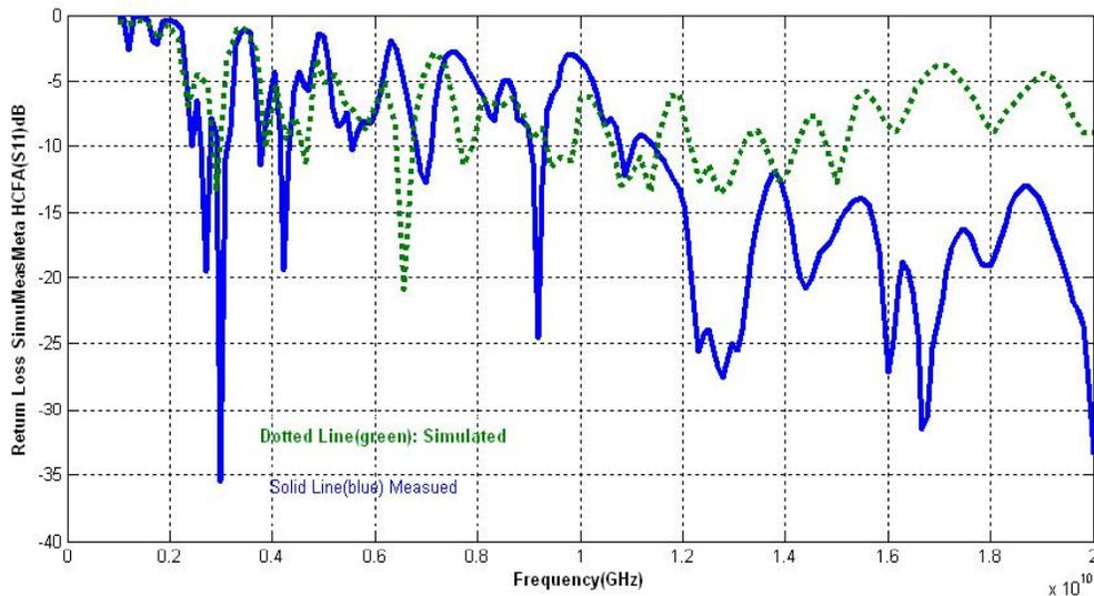
**Figure 7.8 A Comparison of Simulated and Measured Return Loss Characteristics of CSRR Loaded HCFA**
