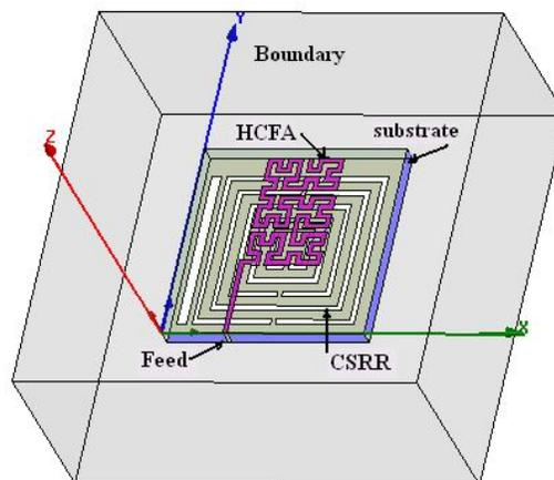
**Figure 7.2 CSRR Loaded HCFA in Simulation**
