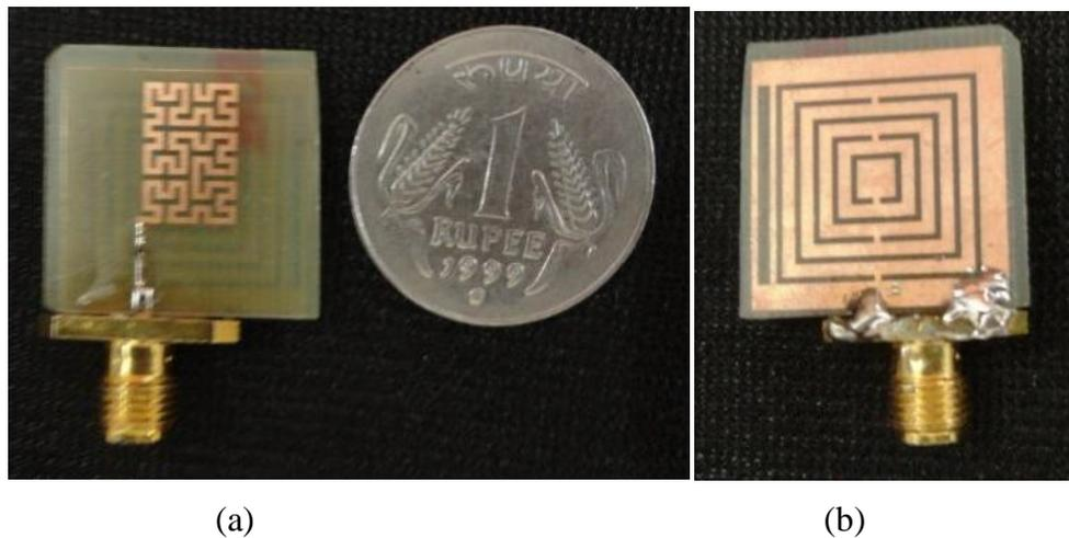
**Figure 7.6 Photographs of Fabricated Antenna (a) Front View of CSRR Loaded HCFA (b) Rear View of Antenna with CSRR**
