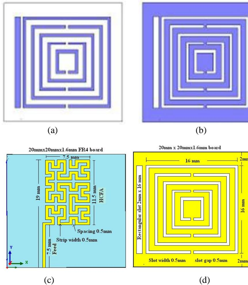
**Figure 7.1** Antenna and MTM Structures (a) MSRR (Blue Colored Lines- Conducting Rings and White Spacing-Substrate) (b) CSRR (White Spacing-Slots - Substrate and Blue Colored Portion-Conducting Part) (c) HCFA (d) CSRR as Defected Ground Plane
