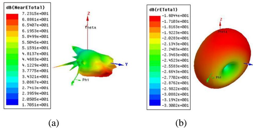
**Figure 6.5 Radiation Patterns of HCFA 1 (Air Environment- Total E Field and 3D Polar Plot) (a) Near Field (At Distance of 10mm) (b) Far-Field**
