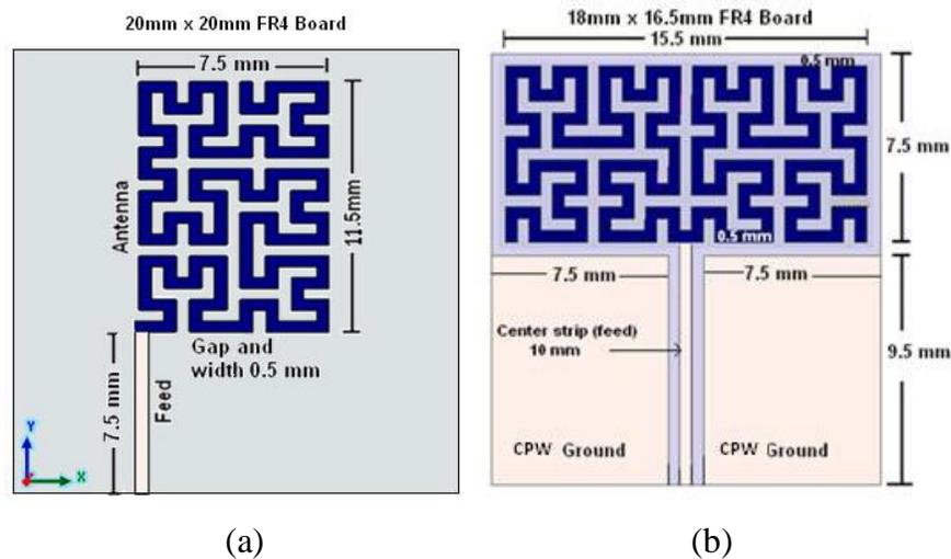
**Figure 6.2 Proposed Antenna Structure (a) HCFA 1 (b) HCFA 2**
