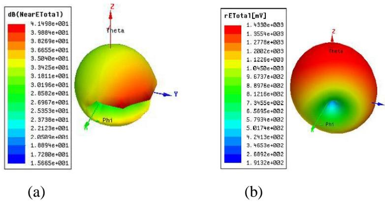
**Figure 6.6 Radiation Patterns of HCFA 1 (Muscle Tissue Environment- Total E Field and 3D Polar Plot (a) Near Field (b) Far-Field**
