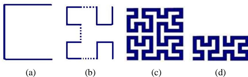
**Figure 6.1 HCFA Antenna Structures (a) Basic Structure (b) Second Iteration (c) Third Iteration (d) Truncated Portion of Third Iteration**
