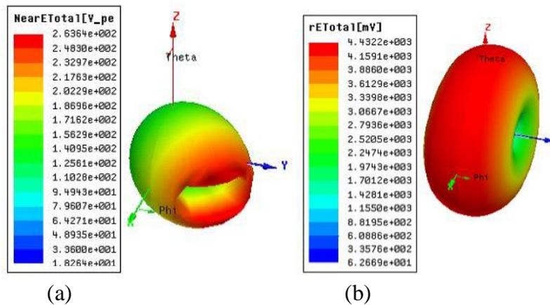
**Figure 6.9 Radiation Patterns of HCFA 2 (Muscle Tissue Environment- Total E Field and 3D Polar Plot) (a) Near Field (At Radius 10mm) (b) Far-Field**
