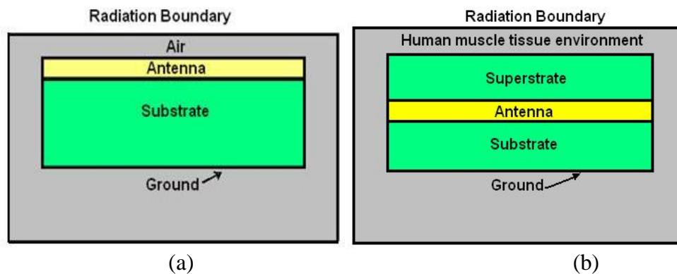
**Figure 6.3 The Different Material Layers of HCFA 1 (a) Different Layers in Air Environment (b) Different Layers in Human Muscle Tissue Environment**
