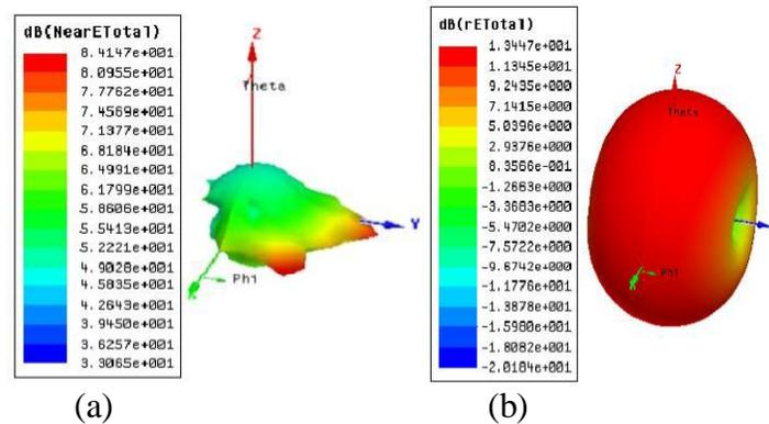
**Figure 6.8 Radiation Patterns of HCFA 2 (Air Environment – Total E Field and 3D Polar Plot) (a) Near Field (At Radius 10mm) (b) Far-Field**
