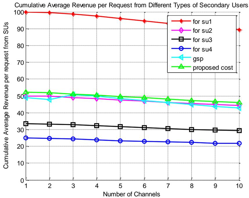
Figure 3.5. Channel allocation cost to different SUs for 50% PU occupancy and medium demand from SUs
