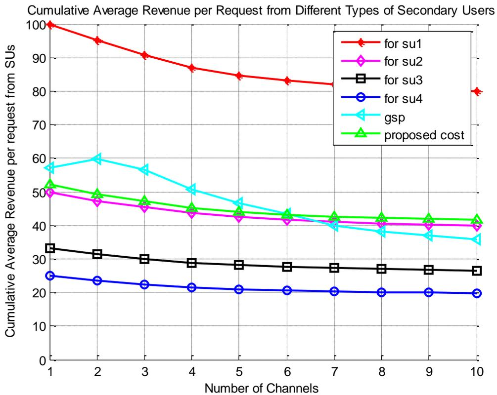
Figure 3.3. Channel allocation cost to different SUs for 25% PU occupancy and low demand from SUs
