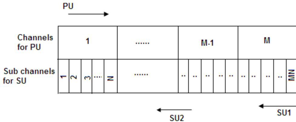
Figure 2.1. System Model of Channel Assignment for Prioritized SUs
