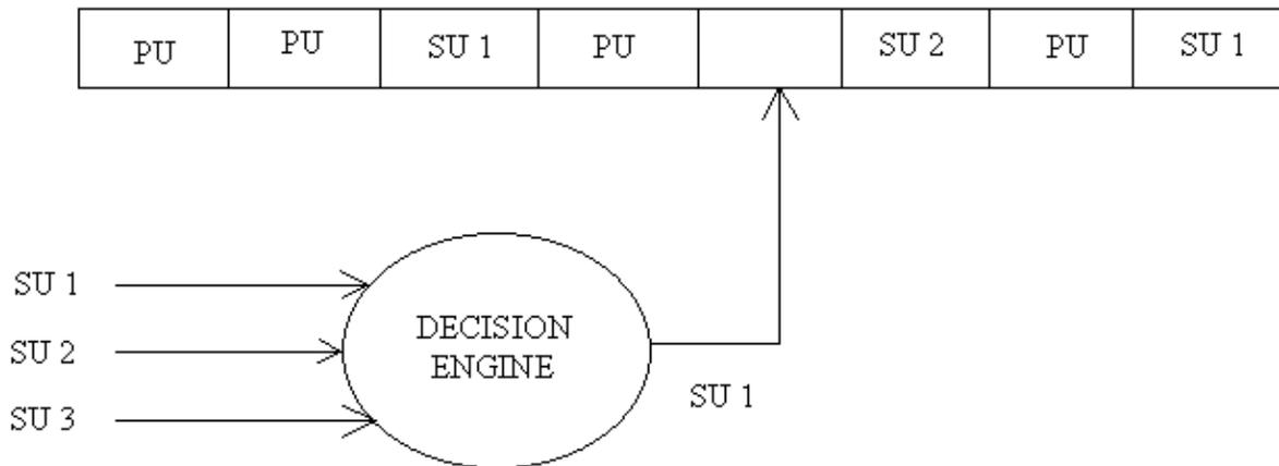
Figure 2.7. Priority based Channel Allocation
