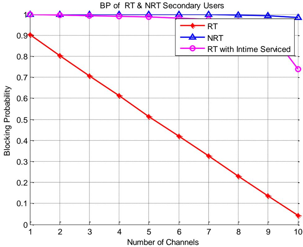
Figure 2.12. Blocking Probability of RT and NRT Secondary Users for High PU Occupancy and High SU Demand
