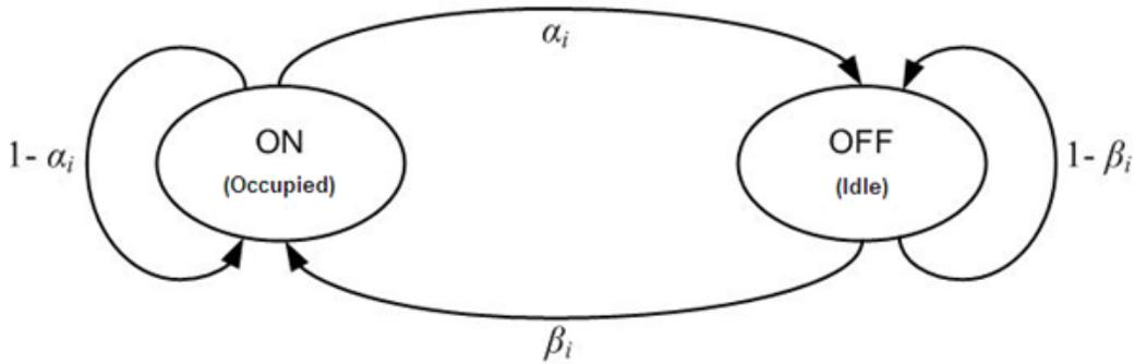
Figure 2.6. Model of channel state
