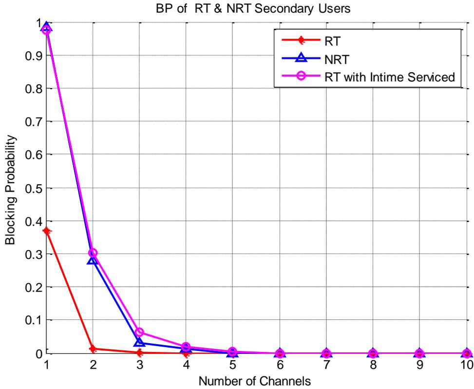
Figure 2.15. Blocking Probability of RT and NRT Secondary Users for High PU Occupancy and Low SU Demand
