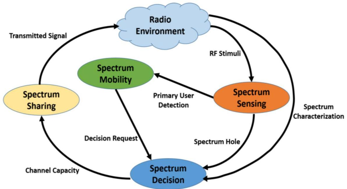
Figure1.4. Life Cycle of Cognitive Radio Network
