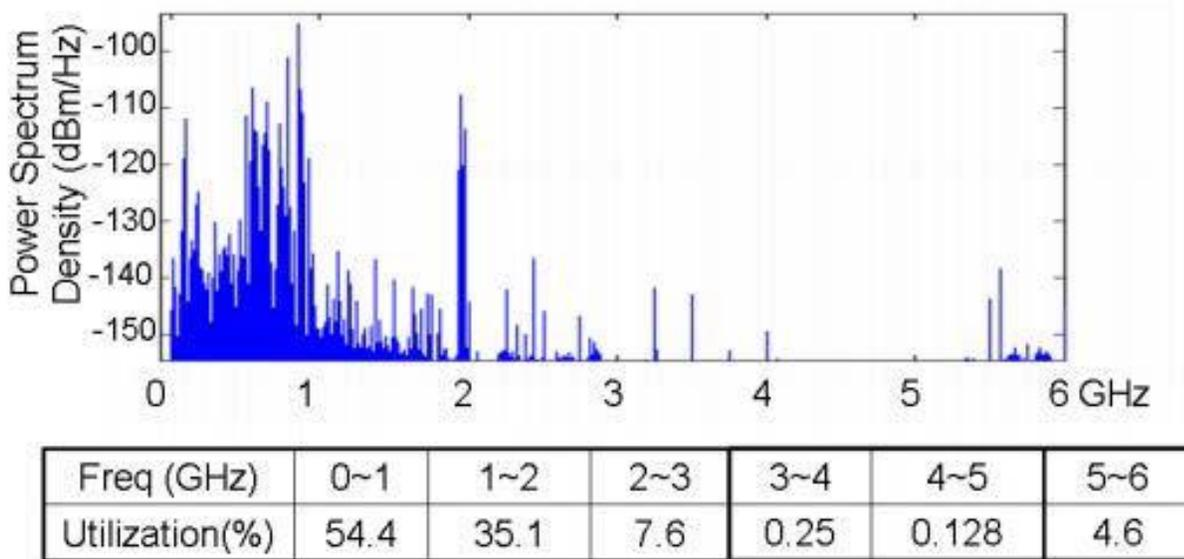
Figure 1.1. Spectrum utilization measurement (0 to 6 GHz) in downtown Berkely
