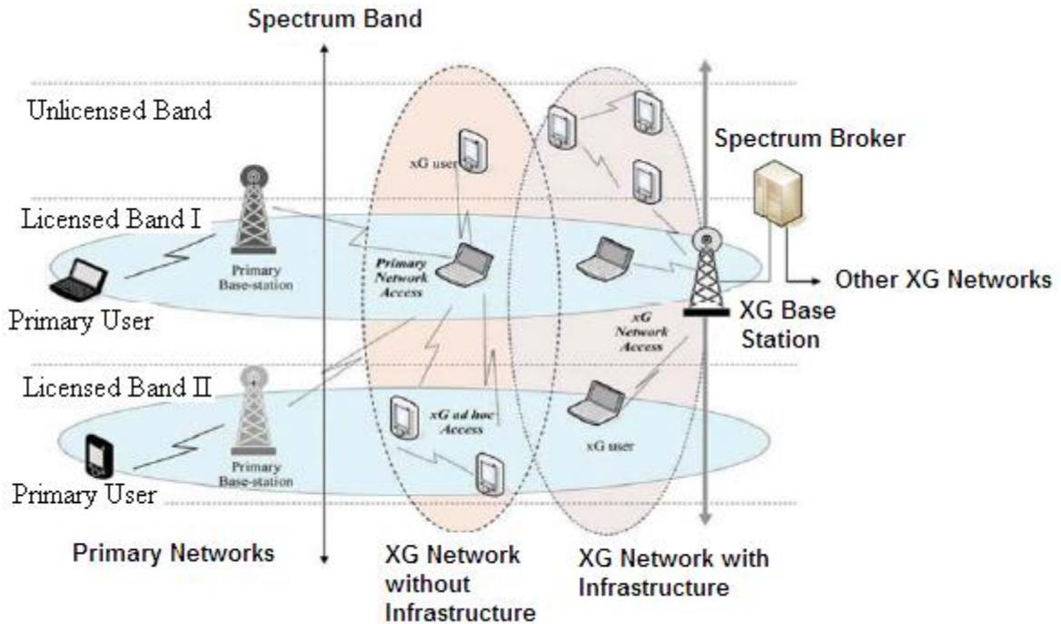
Figure 1.5. Cognitive Radio Network Architecture
