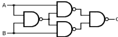
Fig.1.1 Two input Exclusive OR using NAND gates (M. M. Mano, 1979)
