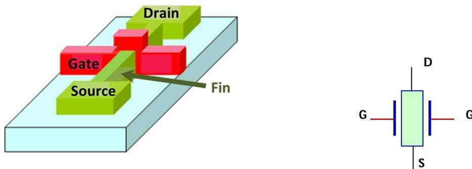
Fig.1.3 Double gate FinFET Structure: Top view and its symbol (D. Bhattacharya et al, 2014)
