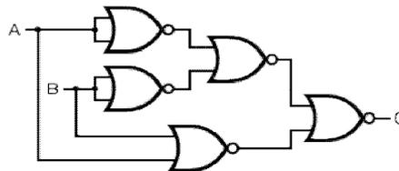
Fig.1.2 Two input Exclusive OR using NOR gates (M. M. Mano, 1979)
