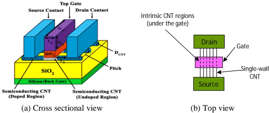
Fig.1.4 Schematic diagram of a CNTFET device (M.H. Moaiyeri et al, 2013)
