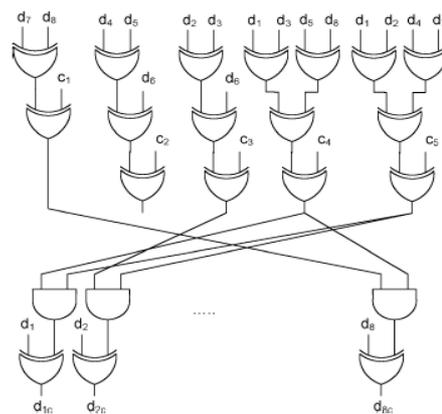
Fig.1.6(a) Low Delay SEC-DED Hamming Encoder (P.Reviriego et al, 2013) Fig.1.6(b) Low Delay SEC-DED Hamming Decoder (P.Reviriego et al, 2013)
