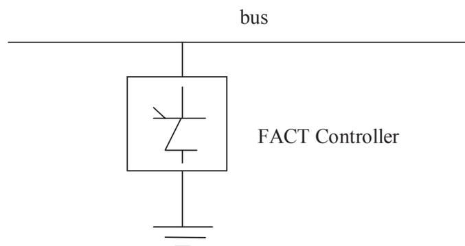
**Fig.1.3 block diagram of shunt compensation**
