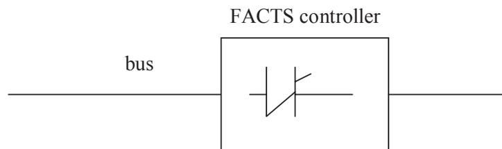
**Fig. 1.4 block diagram of series compensation**
