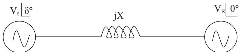
**Figure 1.1 Model of power system**
