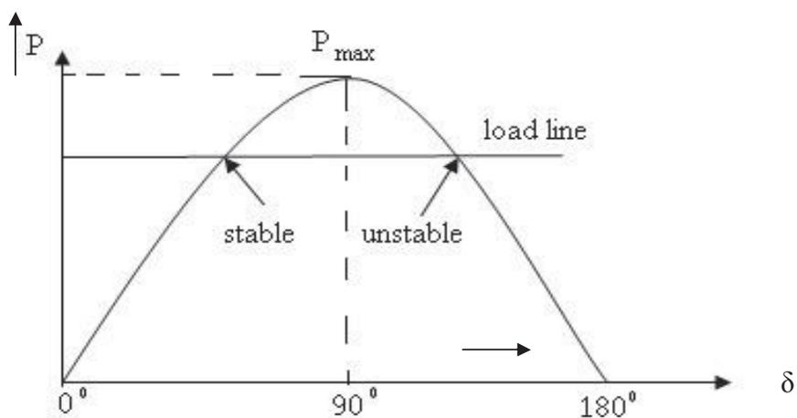
**Figure 1.2 Power angle curve for Figure 1.1**
