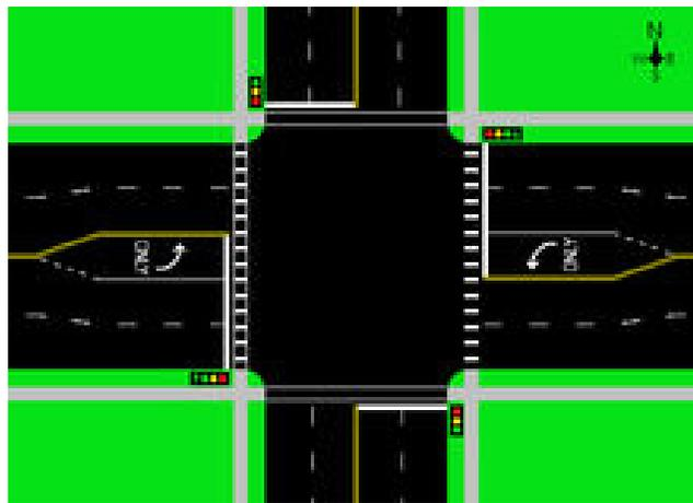
Diagram of an example intersection of two-way streets as seen from above (traffic flows on the right side of the road). The East-West street has left turn lanes from both directions, but the North-South street does not have left turn lanes at this intersection. The East-West street traffic lights also have green left turn arrows to show when unhindered left turns can be made. Some possible markings for crosswalks are shown as examples.
