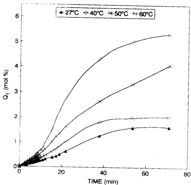
**Figure 7.7.** Effect of temperature on the sorption curves
