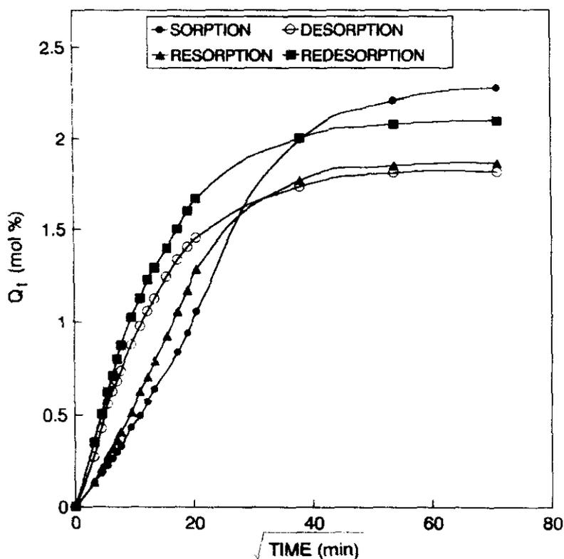
**Figure 7.20.** Sorption-desorption-resorption-redesorption curves of  $N_{50}P$  in carbon tetrachloride
