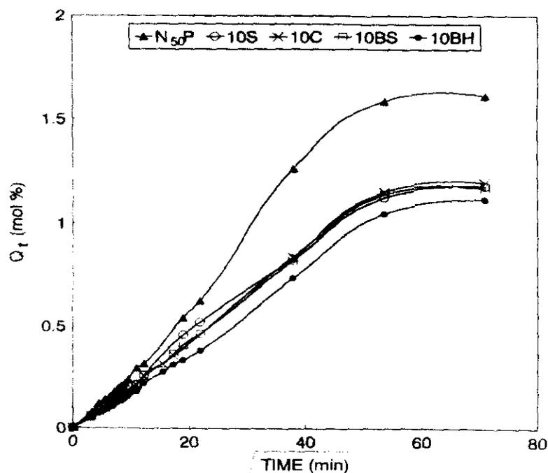
**Figure 7.4.** Sorption curves of unfilled and various filled NBR/EVA blends
