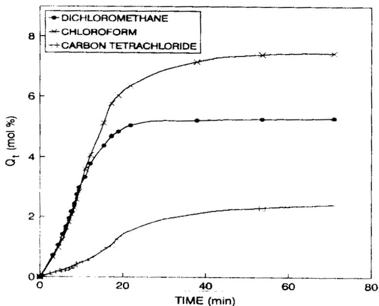
**Figure 7.19.** Sorption curves of  $N_{50}P$  in different solvents
