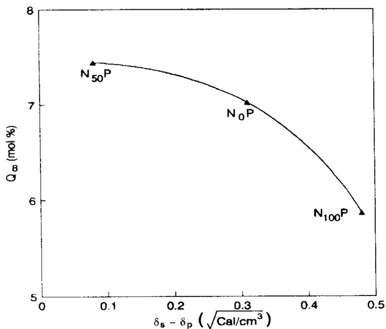
**Figure 7.17.**  $\delta_s - \delta_p$  vs. equilibrium uptake curve for NBR/EVA-chloroform system
