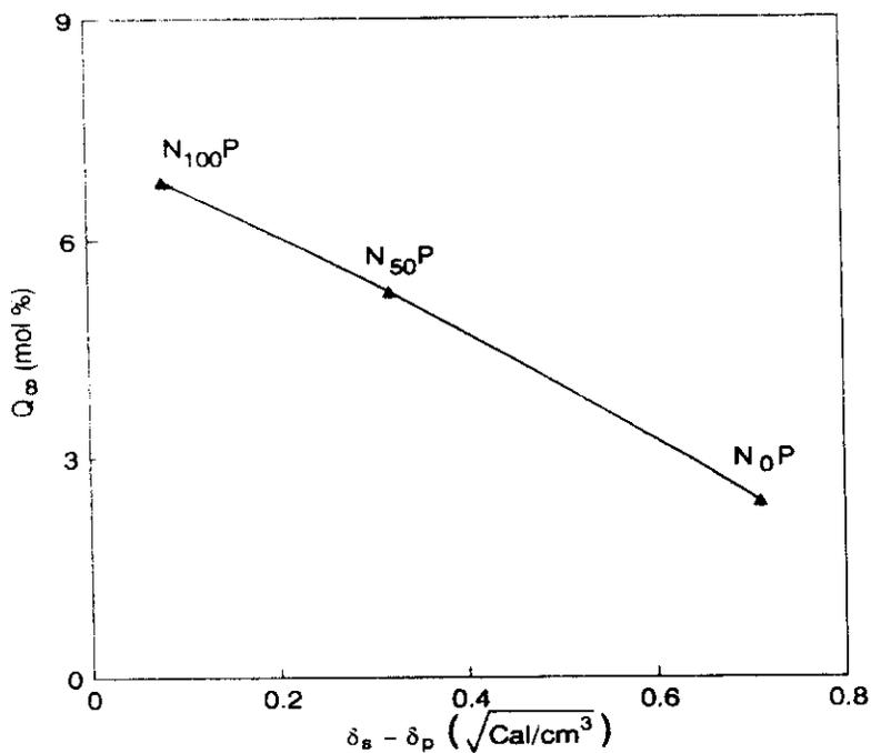
**Figure 7.16.**  $\delta_s - \delta_p$  vs. equilibrium uptake curve for NBR/EVA-dichloromethane system
