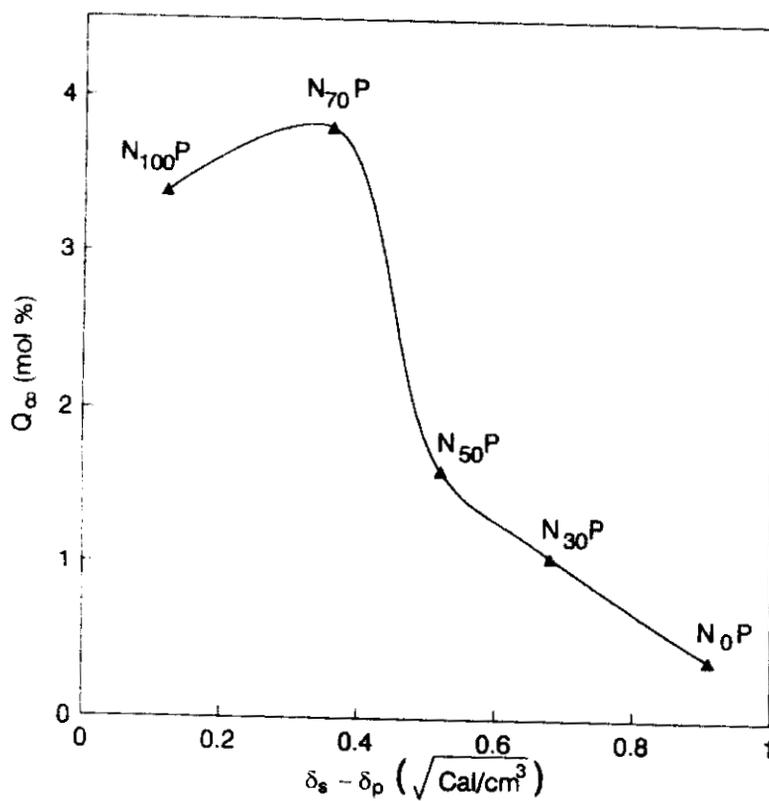
Figure 7.2.  $\delta_s - \delta_p$  vs. equilibrium uptake curve of NBR/EVA-cyclohexanone system
