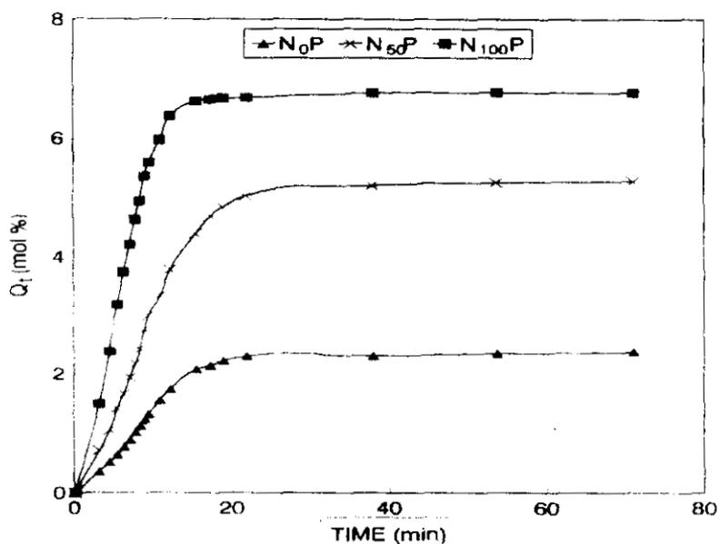
Figure 7.13. Sorption behaviour of NBR/EVA blends in dichloromethane
