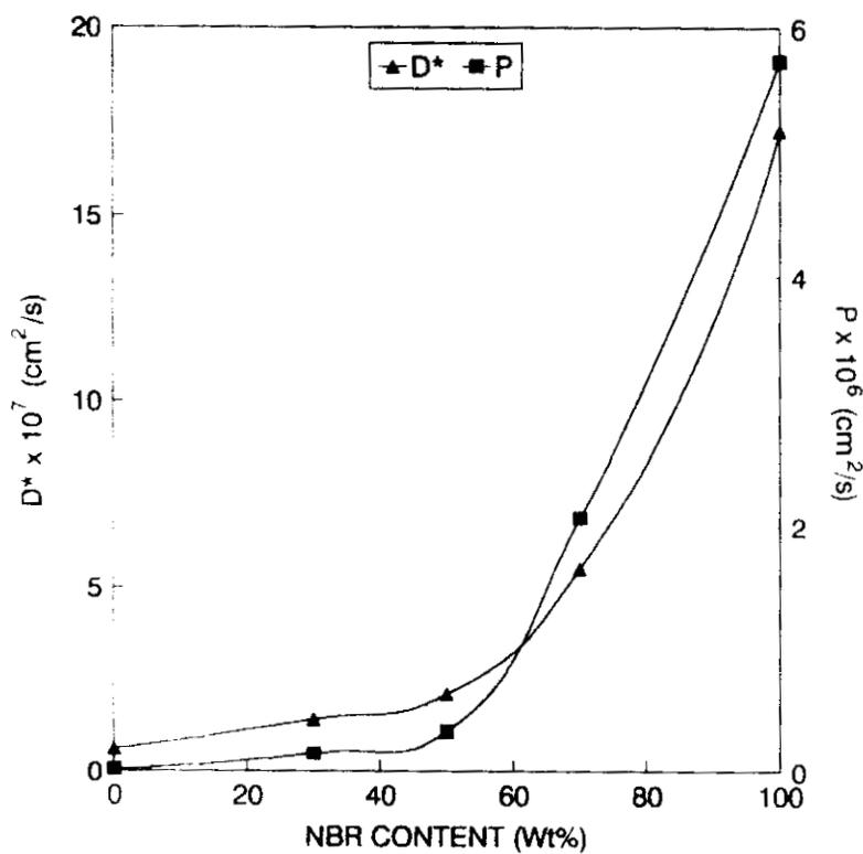
Figure 7.9. Variation of D\* and P with the weight percentage of NBR
