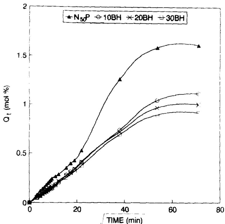
Figure 7.5. Effect of filler loading on the sorption curves
