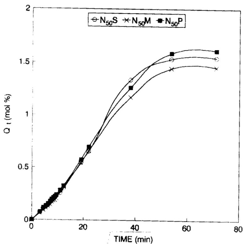
Figure 7.3. Sorption curves of various crosslinked NBR/EVA blends
