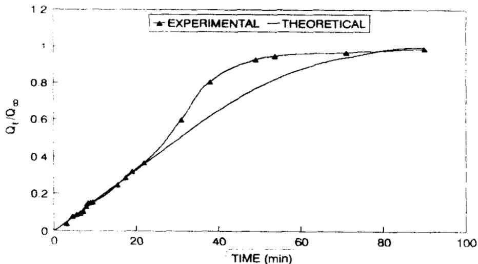
Figure 7.12. Comparison of theoretical and experimental sorption curves
