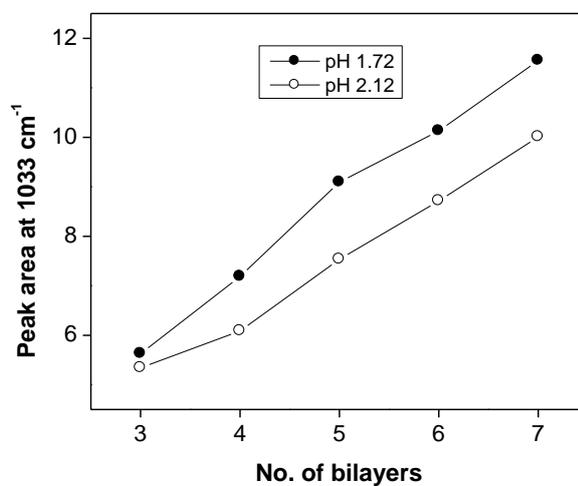
**Figure 3.6:** Area under the sulfonate peak ( $1033\text{ cm}^{-1}$ ) in the FT-IR spectrum as a function of the number of deposited layers at two different pHs 1.72 and 2.12
