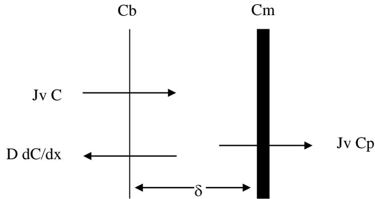
**Figure 3.14:** Mass balance of solute on the membrane boundary layer<sup>32</sup>
