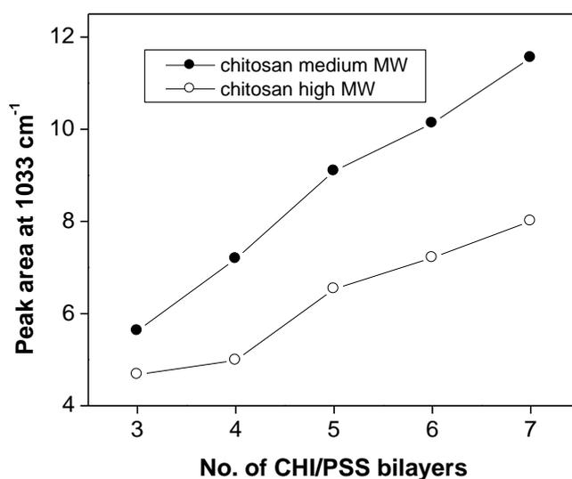
**Figure 3.9:** The peak area at  $1033\text{ cm}^{-1}$  in the FT-IR spectrum as a function of the number of bilayers when multilayers are fabricated from CHI (medium MW) /PSS and CHI (high MW) /PSS
