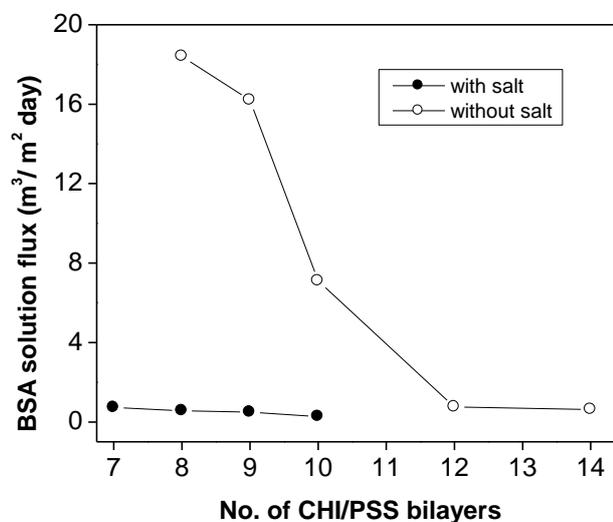
**Figure 3.8:** BSA solution flux as a function of number of CHI/PSS bilayers when the multilayers are fabricated in the presence and the absence of salt.
