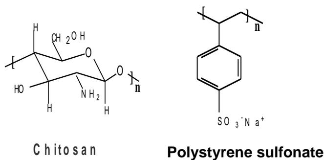
**Figure 3.1:** Polyelectrolytes used for coating
