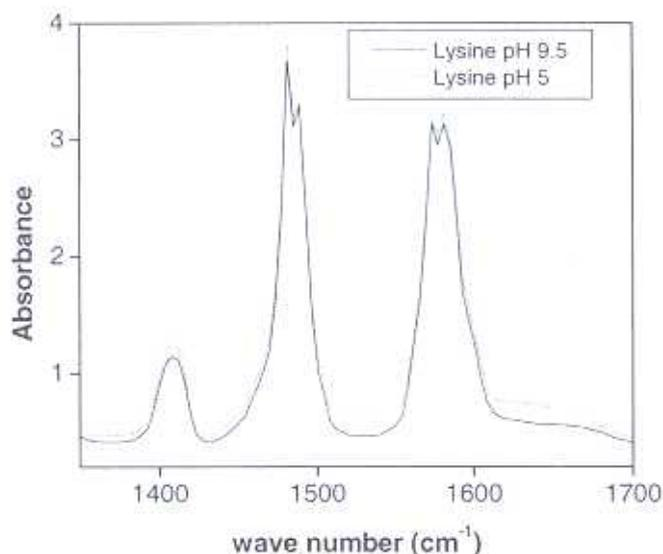
Figure 3.31: FT-IR spectrum of lysine adsorbed on 5 bilayers of CHI/PSS membranes
