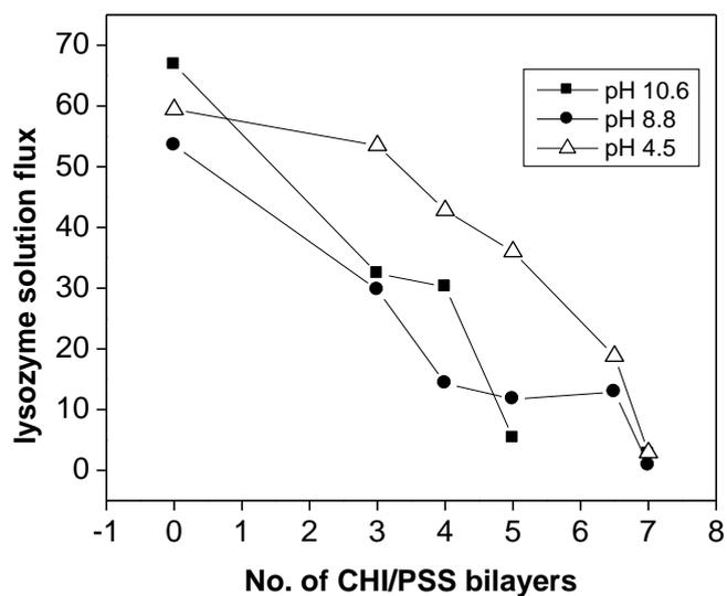
**Figure 3.16:** Lysozyme solution flux as a function of the number of bilayers for lysozyme solutions of different pHs., 10.6, 8.8 and 4.5
