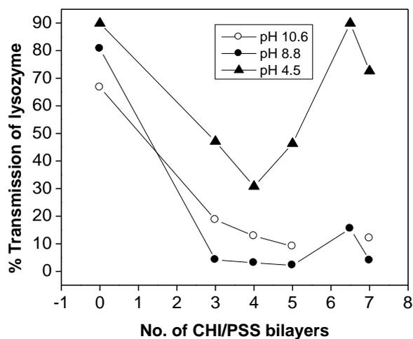
**Figure 3.15:** Percentage transmission of lysozyme as a function of the number of bilayers for lysozyme solutions of different pHs., 10.6, 8.8 and 4.5
