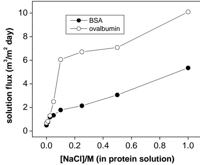
**Figure 3.21:** Solution flux Vs NaCl concentration for BSA and ovalbumin with 9 bl CHI/PSS membrane
