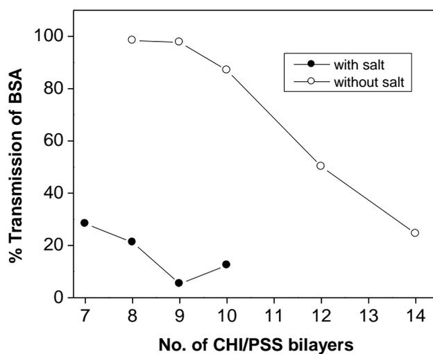
**Figure 3.7:** Percentage transmission of BSA as a function of number of CHI/PSS bilayers when the multilayers are fabricated in the presence and the absence of salt.
