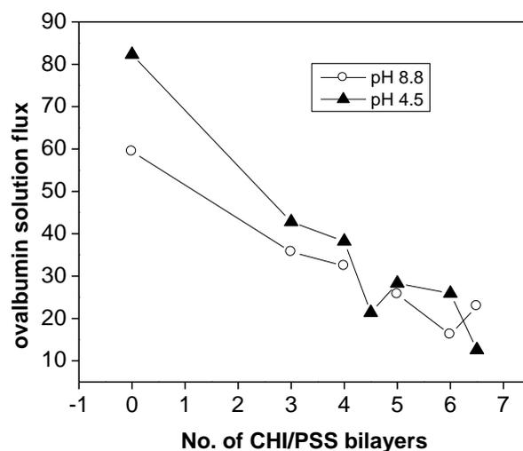
**Figure 3.13:** Ovalbumin solution flux as a function of the number of bilayers for ovalbumin solutions of different pHs, 8.8 and 4.5
