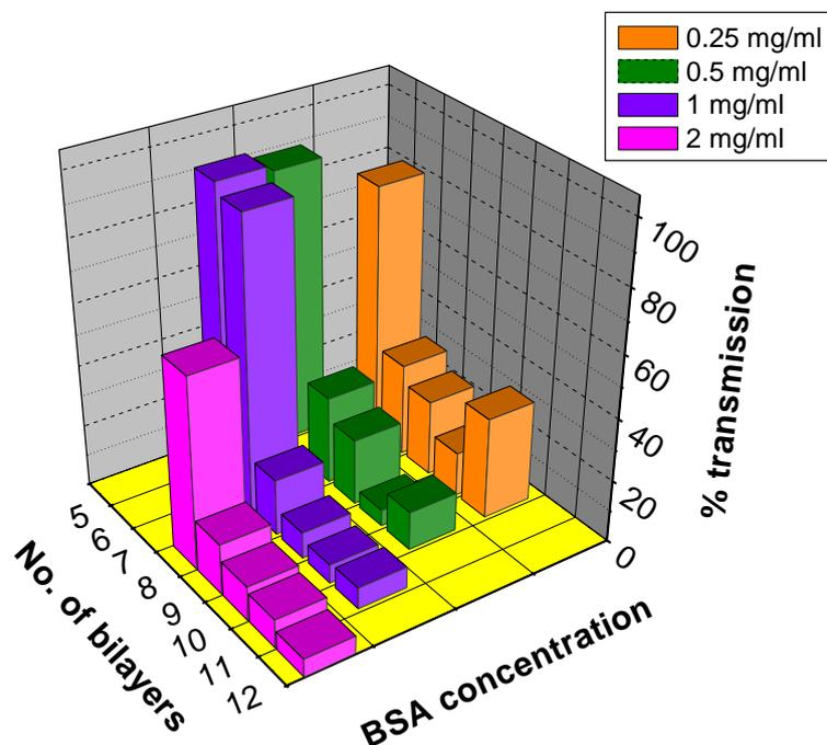
**Figure 3.26:** Transmission profile of BSA of different concentration through CHI/PSS multilayers
