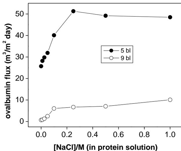
**Figure 3.23:** Comparison of flux and NaCl concentration for ovalbumin through 5 bl and 9 bl CHI/PSS membranes
