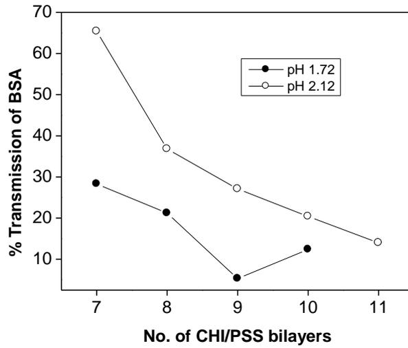
**Figure 3.4:** Percentage transmission of BSA as a function of number of CHI/PSS bilayers when the multilayers are fabricated at two different pHs 1.72 and 2.12.
