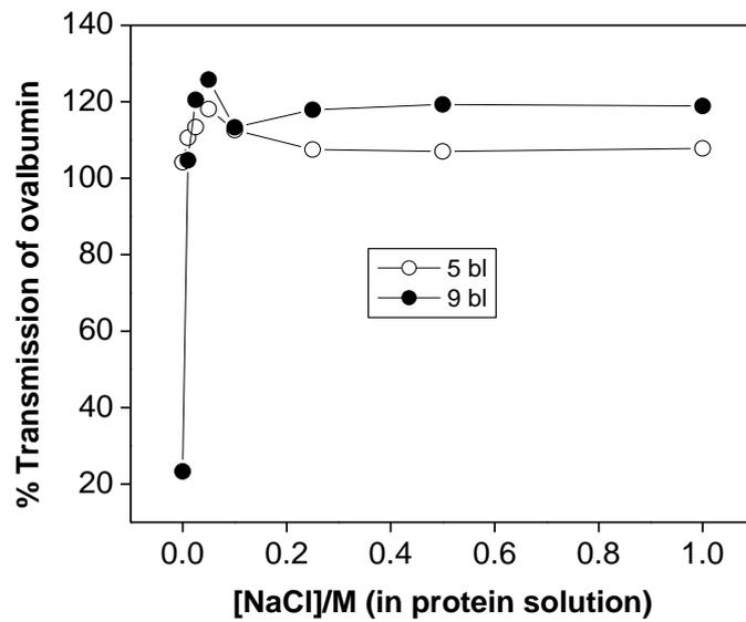
**Fig.3.22:** Comparison of percentage transmission and NaCl concentration for ovalbumin through 5 bl and 9 bl CHI/PSS membranes
