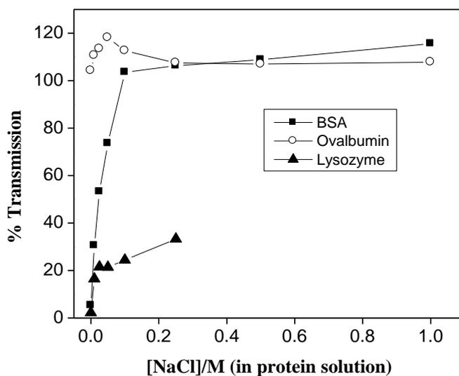
**Figure 3.18:** Effect of ionic strength on the percentage transmission of BSA (0.5 mg/ml, pH 8.8), ovalbumin (0.5 mg/ml, pH 8.8) and lysozyme (0.25 mg/ml, pH 8.8) through CHI/PSS multilayer membranes. BSA transport studies were carried out with 9 bl system; ovalbumin and lysozyme transport studies were carried out with 5 bl CHI/PSS system
