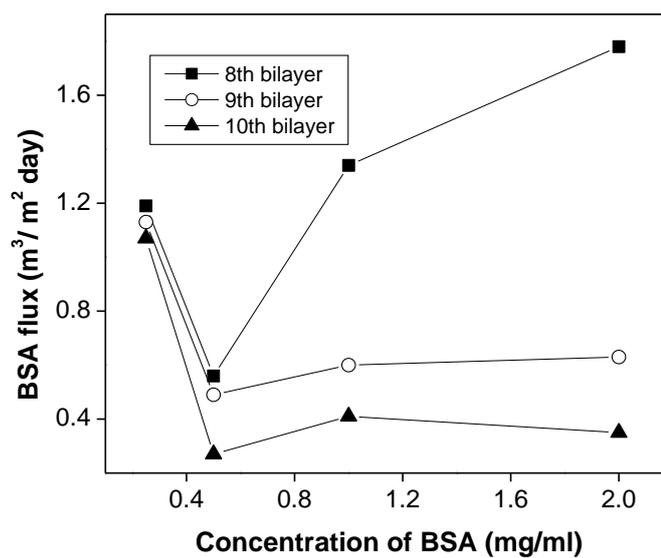
**Figure 3.25:** BSA flux Vs Concentration of BSA (CHI/PSS 8<sup>th</sup>, 9<sup>th</sup>, 10<sup>th</sup> bilayer)
