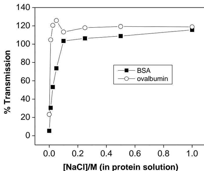
**Figure 3.20:** Percentage transmission Vs NaCl concentration for BSA and ovalbumin with 9 bl CHI/PSS membrane
