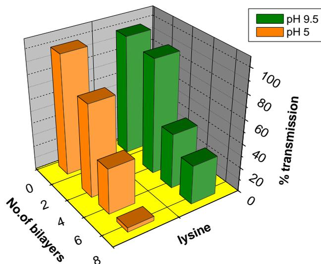
**Figure 3.30:** Transmission profile of L-lysine through CHI/PSS multilayer membrane
