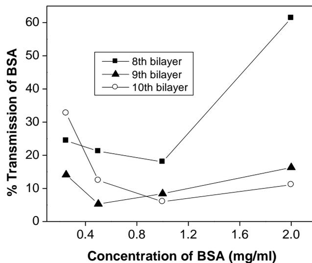
**Figure 3.24:** Percentage transmission of BSA Vs Concentration of BSA (CHI/PSS 8<sup>th</sup>, 9<sup>th</sup>, 10<sup>th</sup> bilayer)
