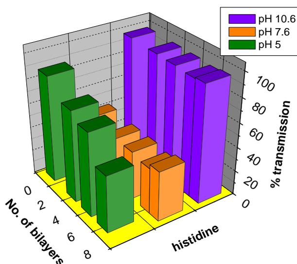
**Figure 3.28:** Transmission profile of L-histidine through CHI/PSS multilayer membrane
