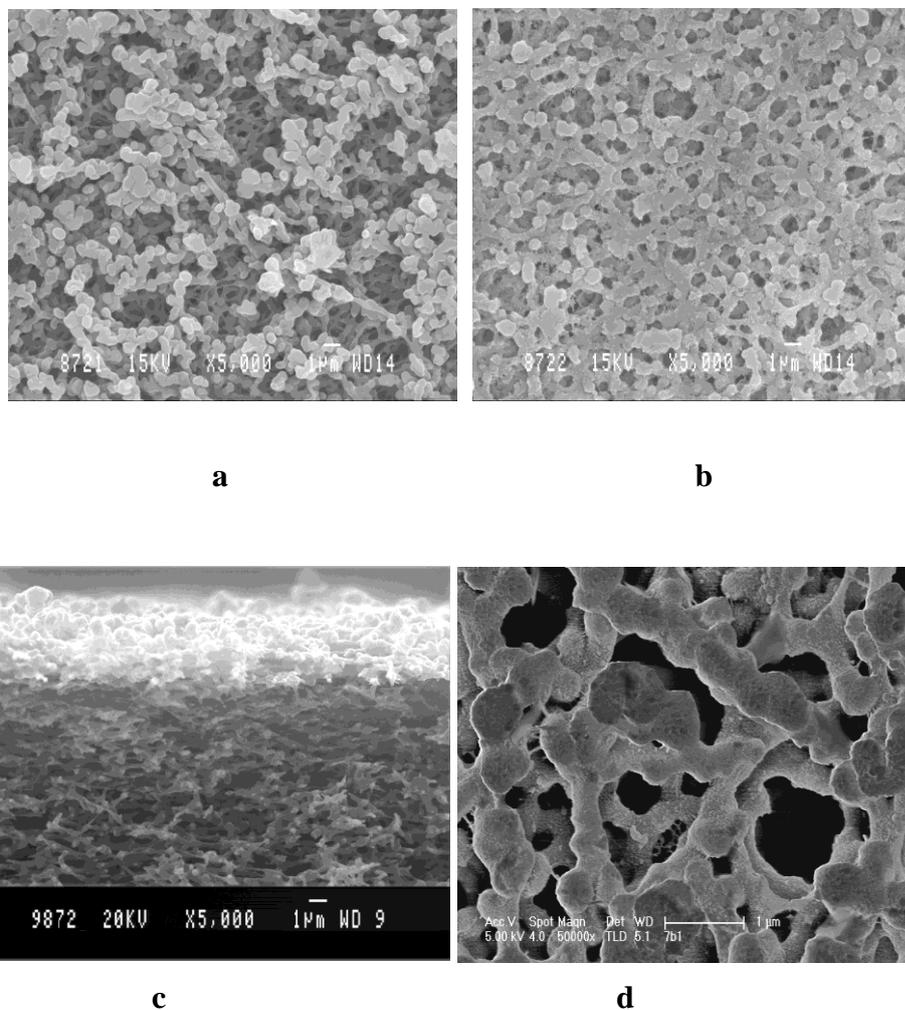
**Figure 3.2:** SEM images of supor and 7 bilayer CHI/PSS membranes [**a:** bare membrane, **b:** 7 bl CHI/PSS coated membrane, **c:** cross-section of 7 bl CHI/PSS membrane, **d:** 7 bl CHI/PSS (0.1 M NaCl) membrane]
