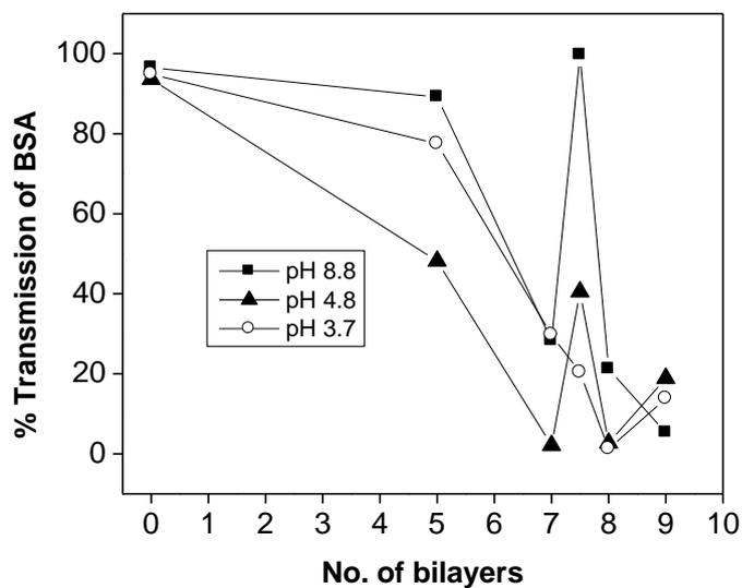
**Figure 3.10:** Percentage transmission of BSA as a function of the number of bilayers for BSA solutions of different pHs., 8.8, 4.8 and 3.7
