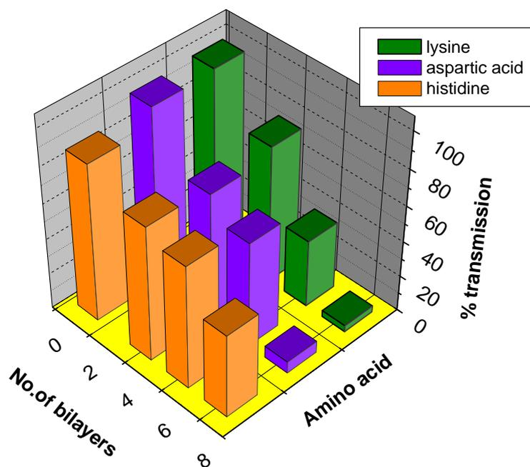
**Figure 3.33:** Transmission profile of lysine, aspartic acid and histidine through CHI/PSS multilayer membrane at pH 5
