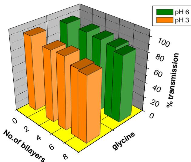
**Figure 3.29:** Transmission profile of glycine through CHI/PSS multilayer membrane
