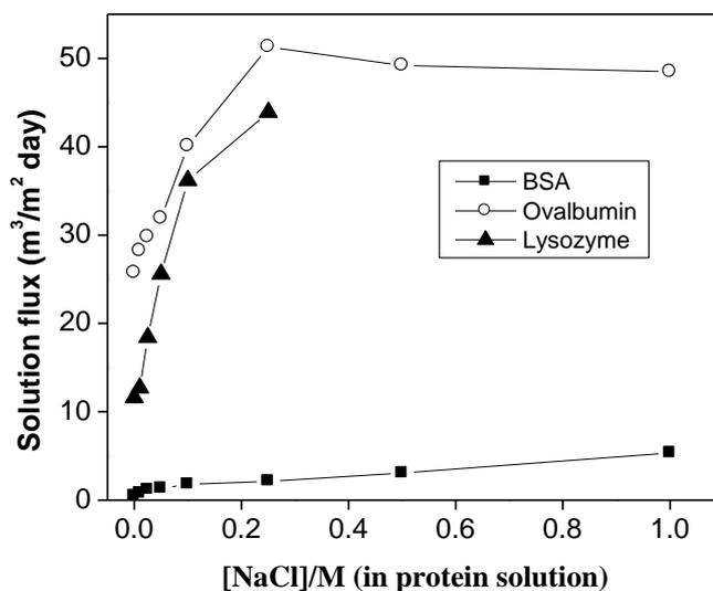
**Figure 3.19:** Effect of ionic strength on the solution flux of BSA (0.5 mg/ml, pH 8.8), ovalbumin (0.5 mg/ml, pH 8.8) and lysozyme (0.25 mg/ml, pH 8.8) through CHI/PSS multilayer membranes. BSA transport studies were done with 9 bl system; ovalbumin and lysozyme transport studies were done with 5 bl CHI/PSS system
