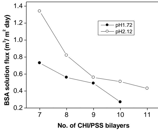
**Figure 3.5:** BSA solution flux as a function of number of CHI/PSS bilayers when the multilayers are fabricated at two different pHs 1.72 and 2.12.
