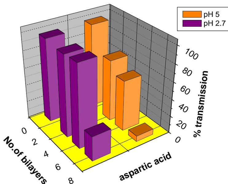
**Figure 3.32:** Transmission profile of L-aspartic acid through CHI/PSS multilayer membrane
