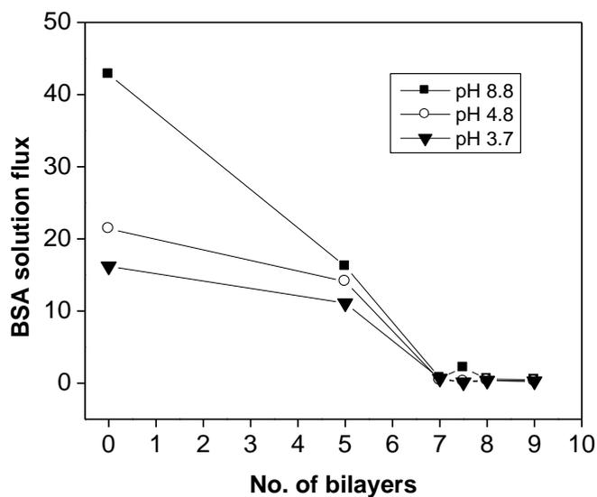
**Figure 3.11:** BSA solution flux as a function of the number of bilayers for BSA solutions of different pHs., 8.8, 4.8 and 3.7
