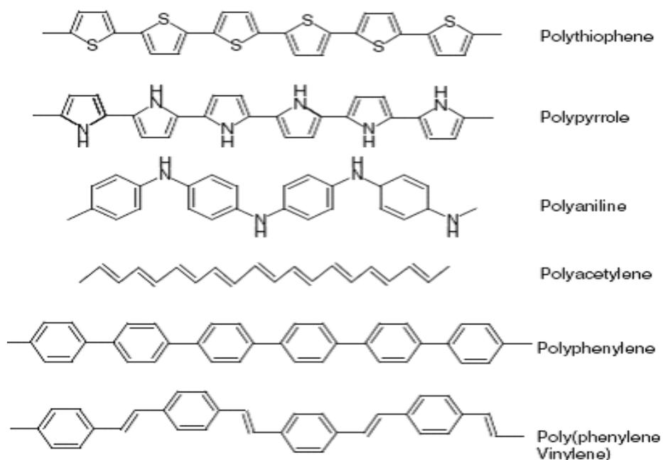
**Fig.1.14:** Structure of conjugated polymers
