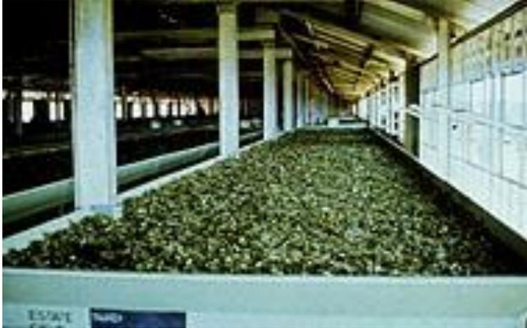
**Fig. 1.3:** Process of Withering
