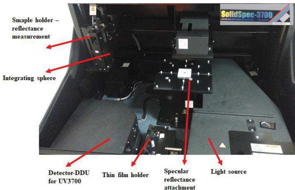
**Figure 2.12.** Major components of UV-Vis spectrophotometer (SolidSpec-3700) instrument.
