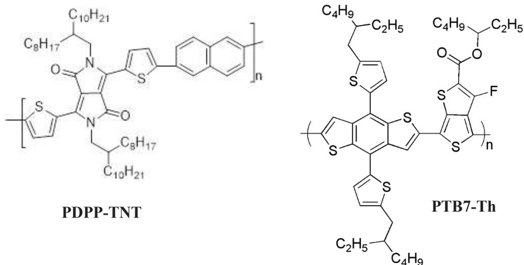
**Figure 2.1.** The molecular structure of low band gap D-A type copolymers used for OPV devices.
