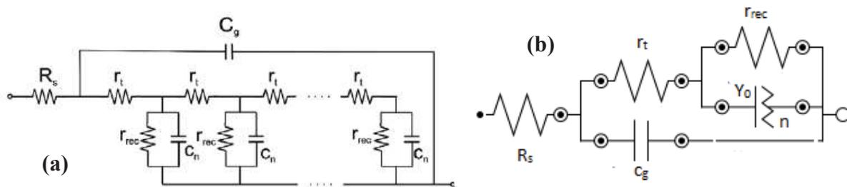
**Figure 2.9.** (a) Infinite series equivalent circuit model and (b) CPE equivalent circuit model
