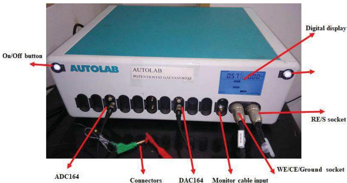
**Figure 2.8.** Autolab (Model No. PGSTAT-302N) impedance analyzer.
