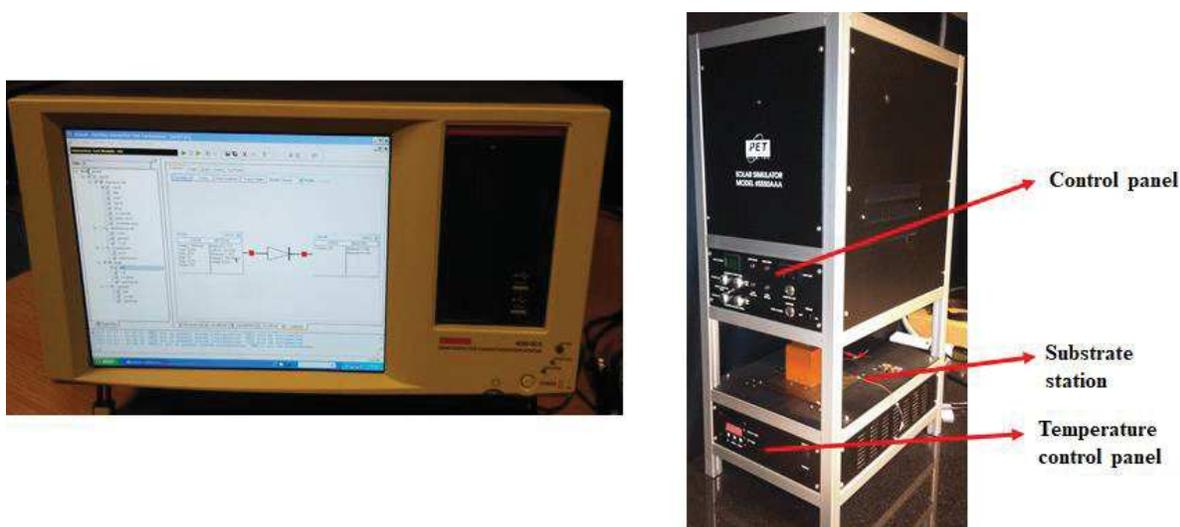
**Figure 2.5.** (a) Keithley semiconductor parameter analyzer set-up, and (b) Solar simulator.
