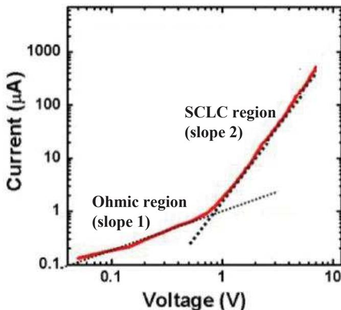
**Figure 2.7.** SCLC behaviour of polymer semiconductor with Ohmic and SCLC regions.
