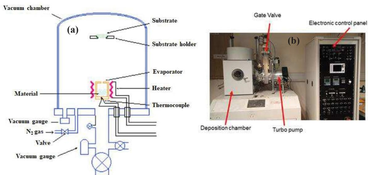
**Figure 2.4.** (a) Schematic of thermal evaporation unit<sup>148</sup>, and (b) Thermal evaporation instrument set-up.
