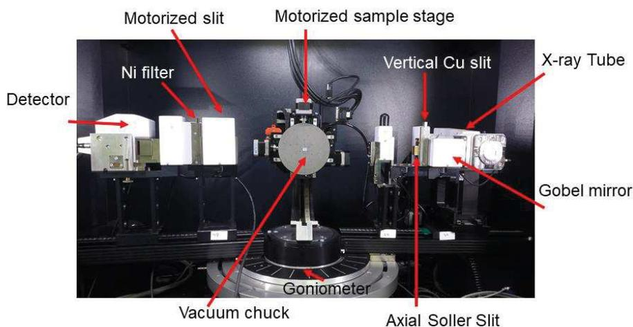
**Figure 2.13.** Image of glancing angle X-ray diffractometer (Bruker, D8-Discover).
