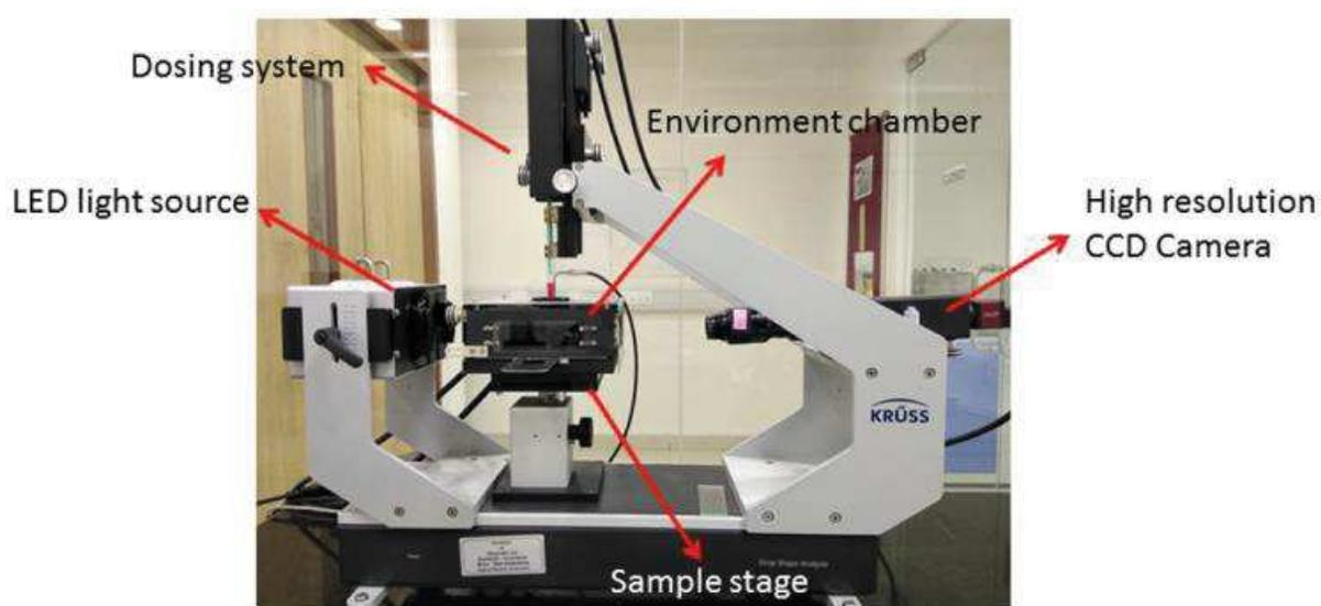
**Figure 2.10.** Photograph of contact angle measurement setup (Krüss, DSA25) with all accessories.
