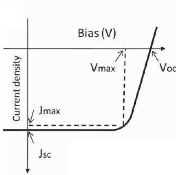
**Figure 2.6.** Current-density vs bias plot for typical solar cell under light along width basic defining parameters of the device.<sup>149</sup>
