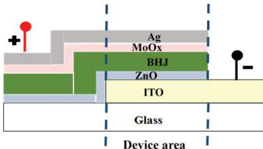
**Figure 2.2.** Device architecture of inverted BHJ OPV solar cells.
