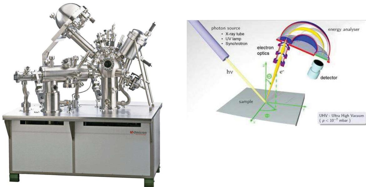
**Figure 2.14.** Photograph of X-ray photoelectron spectroscopy system along with schematic diagram.
