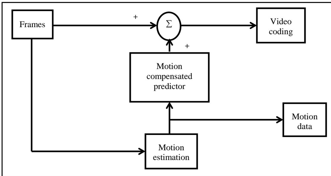
**Figure 3.8: Motion Estimation and Compensation Model for Video Coding**
