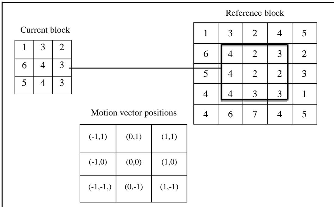
**Figure 3.1: Example for Block-Based Motion Estimation**
