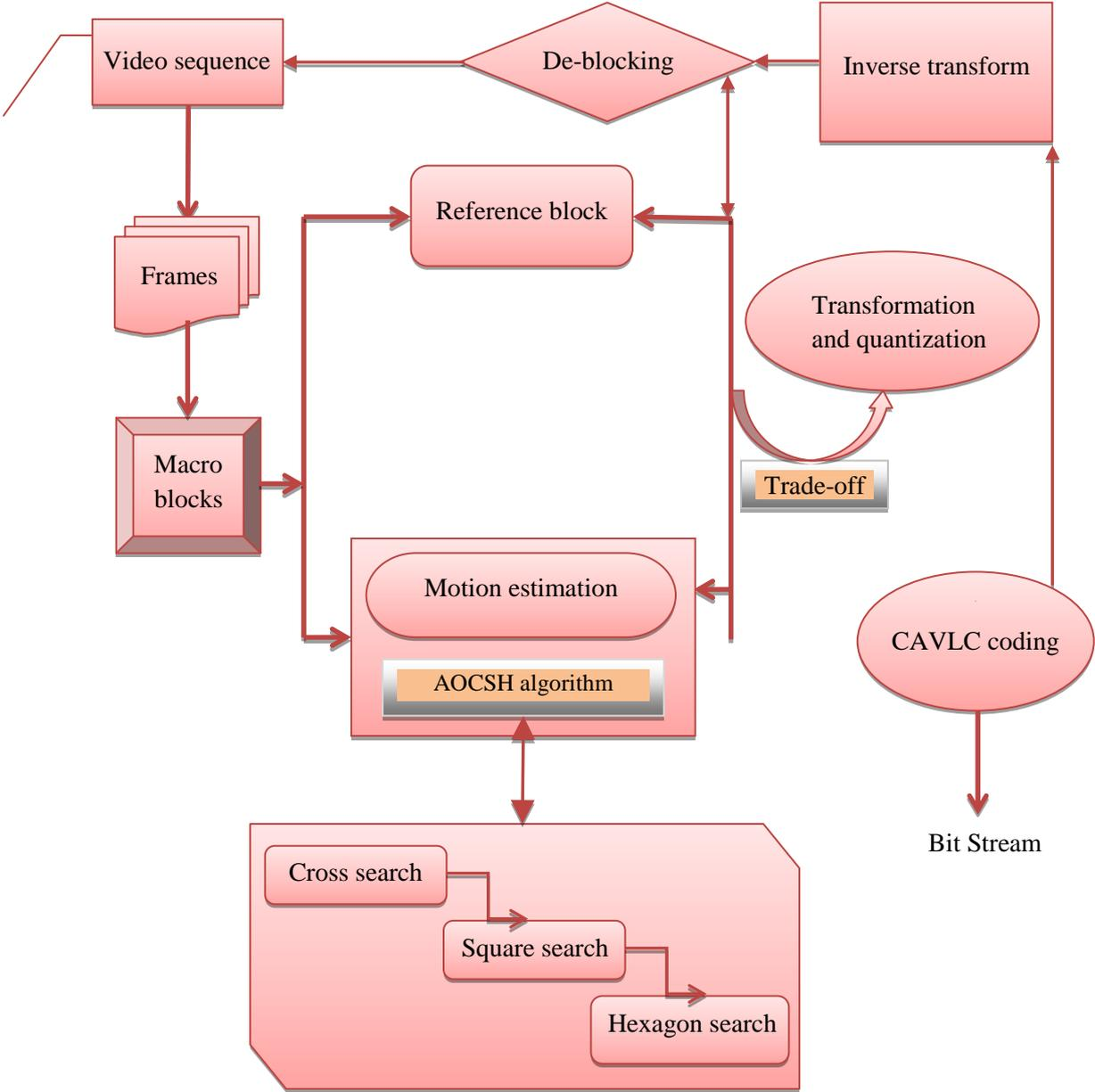
**Figure 5.1: Overall Block Diagram of the AOC SH Motion Estimation Scheme**
