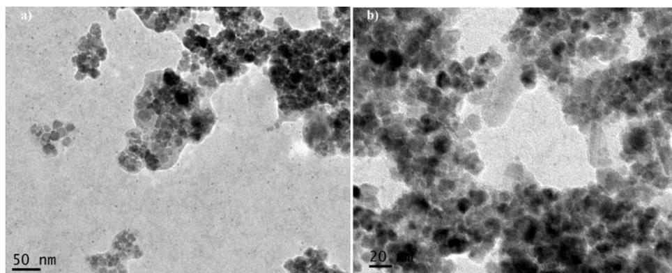
Figure 5.4: TEM images of NP-BBN-SAN complexes with scale bar a) 50 nm and b) 20 nm.
