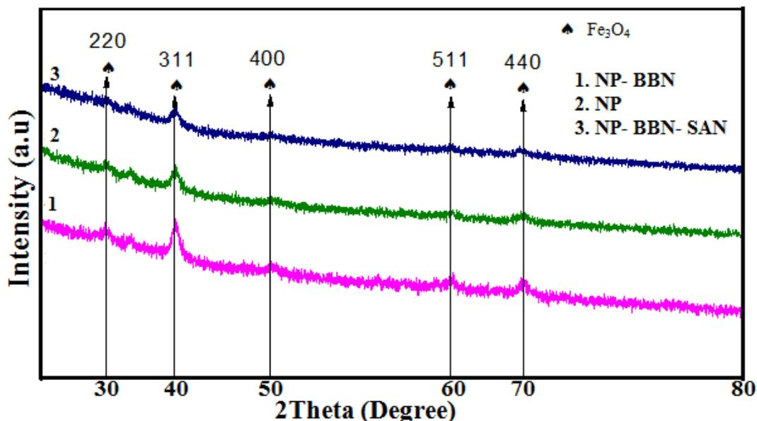
Figure 5.3: XRD pattern of NPs and its complexes with BBN and BBN-SAN.
