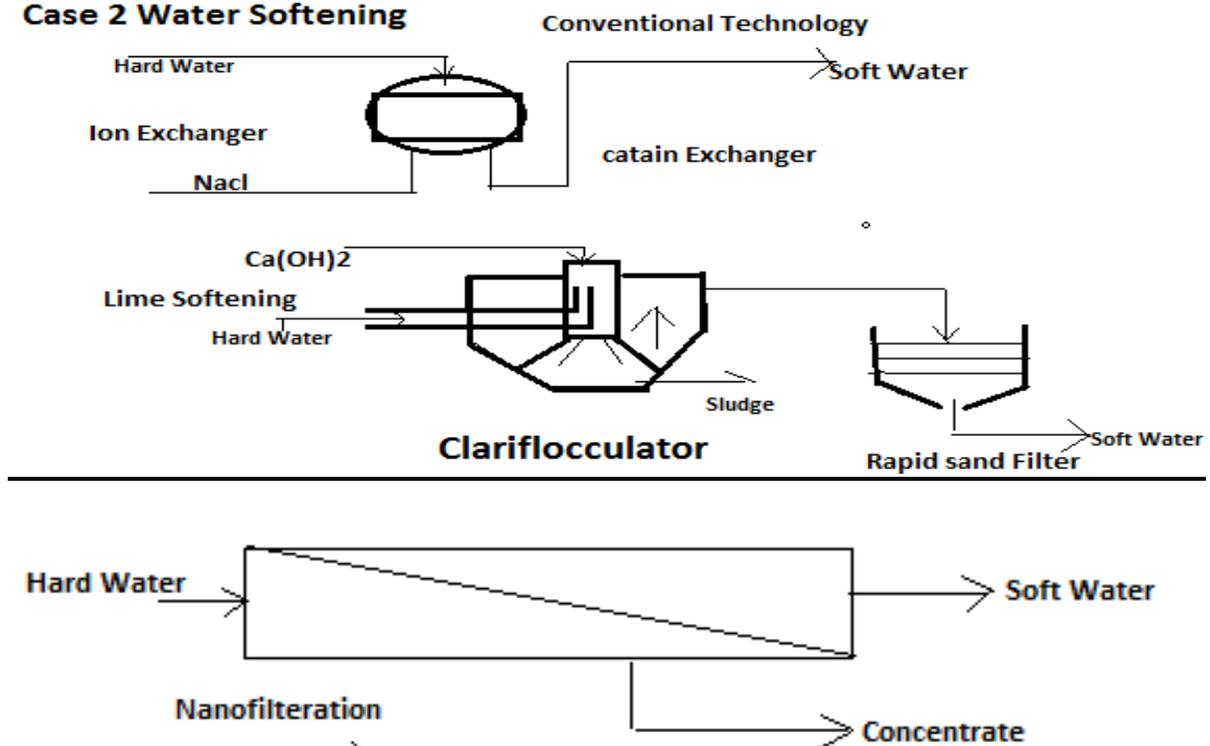
**Figure: 4.10 Water Treatment Through Nanofiltration**
