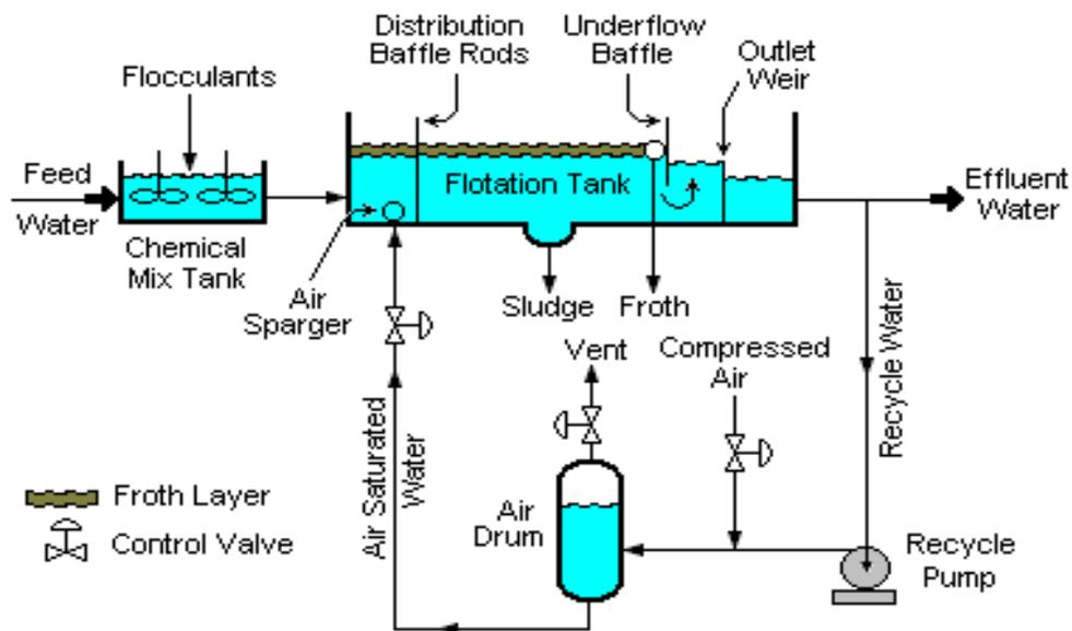
**Figure: 4.4 A typical dissolved air flotation unit [DAF]**
