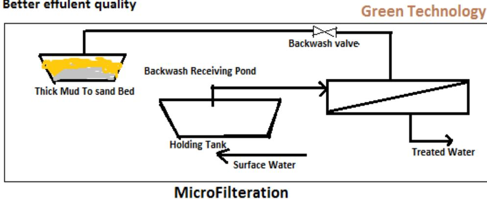
**Figure: 4.9 Water Treatment Through Microfiltration.**
