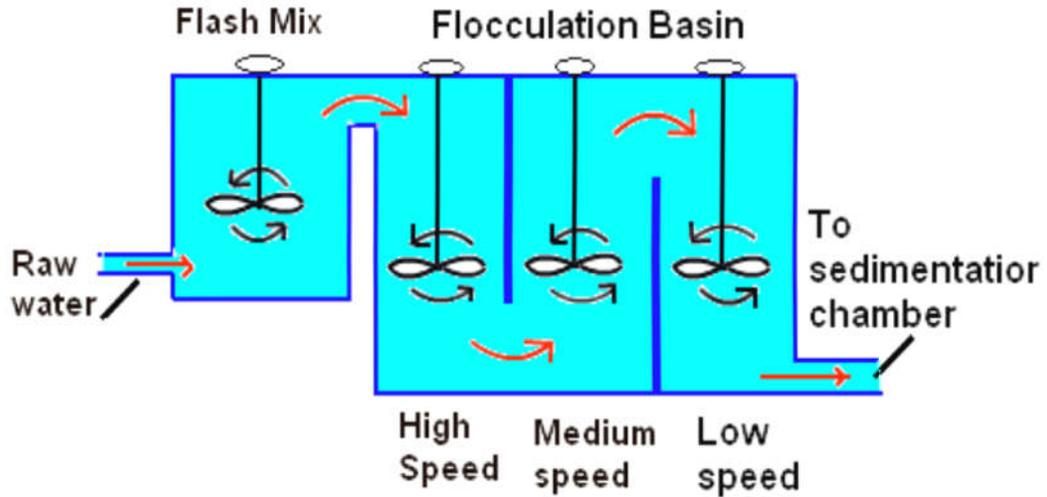
**Figure: 4.2. Flocculation Tank**
