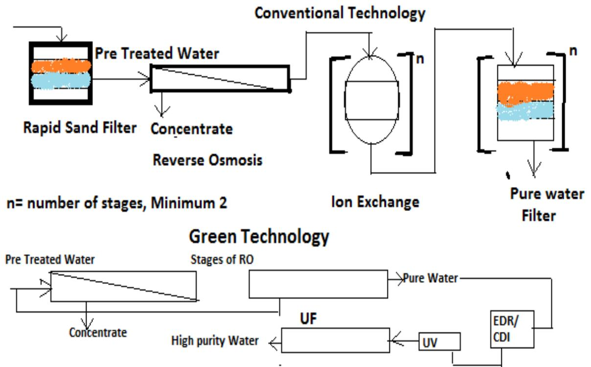
**Figure : 4.11 Water Filtration through Ultra filtration and Reverse Osmosis.**
