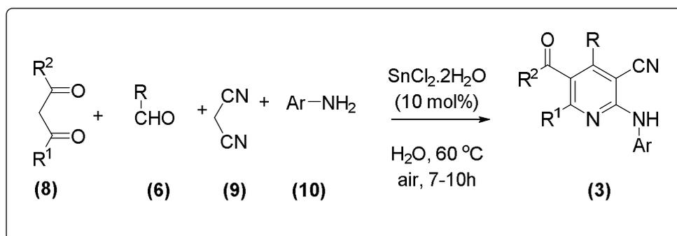
**Scheme 2:** SnCl<sub>2</sub>·2H<sub>2</sub>O catalyzed synthesis of 2-arylamino-3-cyanopyridine derivatives.
