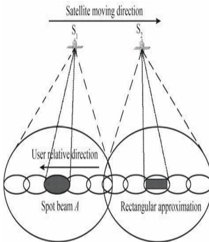
**Fig 1.5:** Spot Beams of Moving Satellite and its Rectangular Approximation
