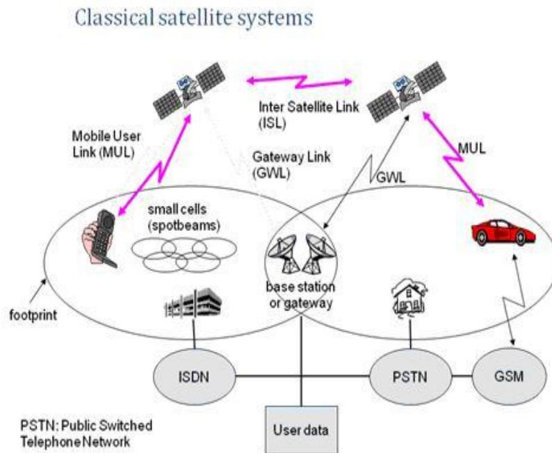
Fig 1.4: Satellite Communication Architecture
