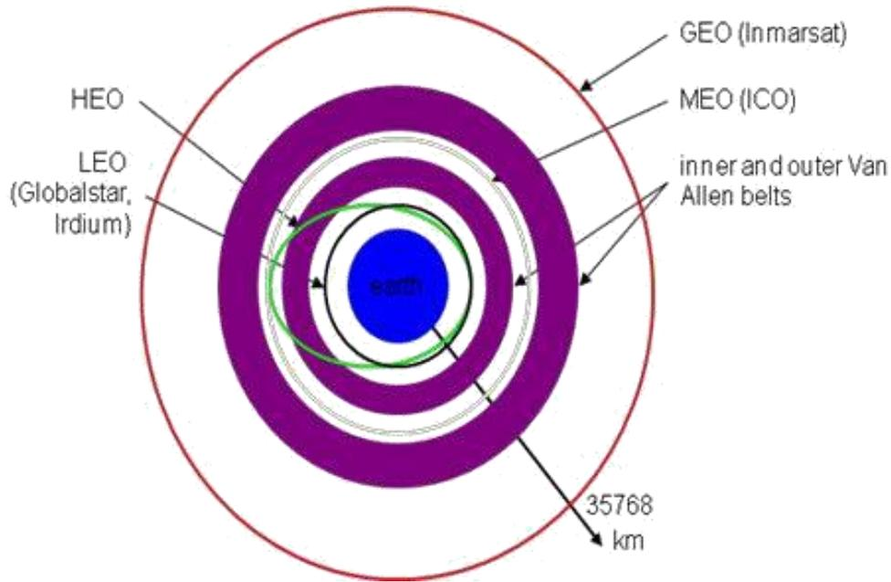
**Fig 1.6:** Diagrammatic Representation of Satellite Orbit
