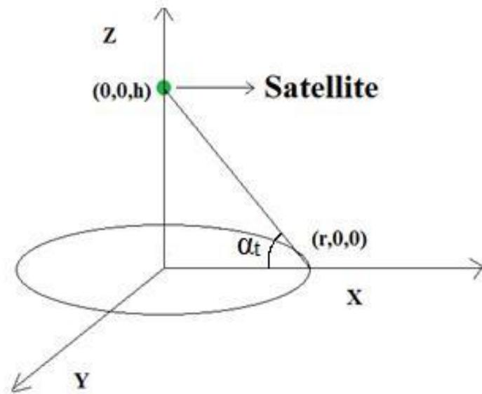
Fig. 5.2: Simplistic situation showing the threshold angle between the satellite and MS
