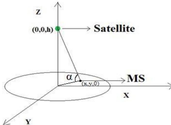
Fig. 5.1: A simplistic situation showing the angle between the satellite and MS
