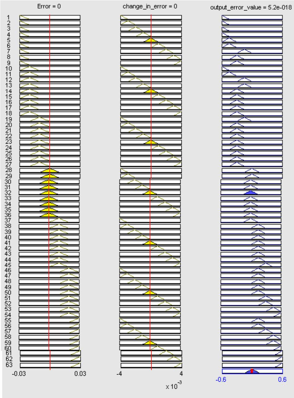
**Figure 4.3 Rule View with defuzzification to represent the change in error to be normalized within the Universe of Discourse**
