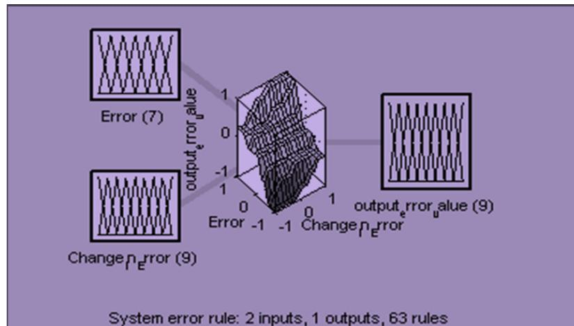
**Figure 4.2 Structure of FIS for detection and correction of error**
