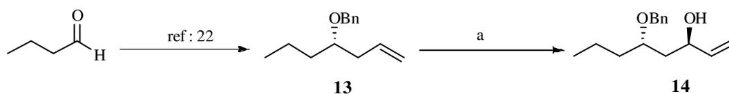
**Scheme 4.** Reagents and conditions. (a) (i) OsO<sub>4</sub>, NaIO<sub>4</sub>, 2,6-lutidine, 1,4-dioxane:H<sub>2</sub>O (3:1), rt, 4.5h; (ii) vinyl magnesium bromide, dry THF, -20 °C, 1h, 75%; (iii) (+)-DIPT, Ti(O<sup>i</sup>Pr)<sub>4</sub>, CHP, 4 Å MS, dry CH<sub>2</sub>Cl<sub>2</sub>, -20 °C, 12h, 45%.
