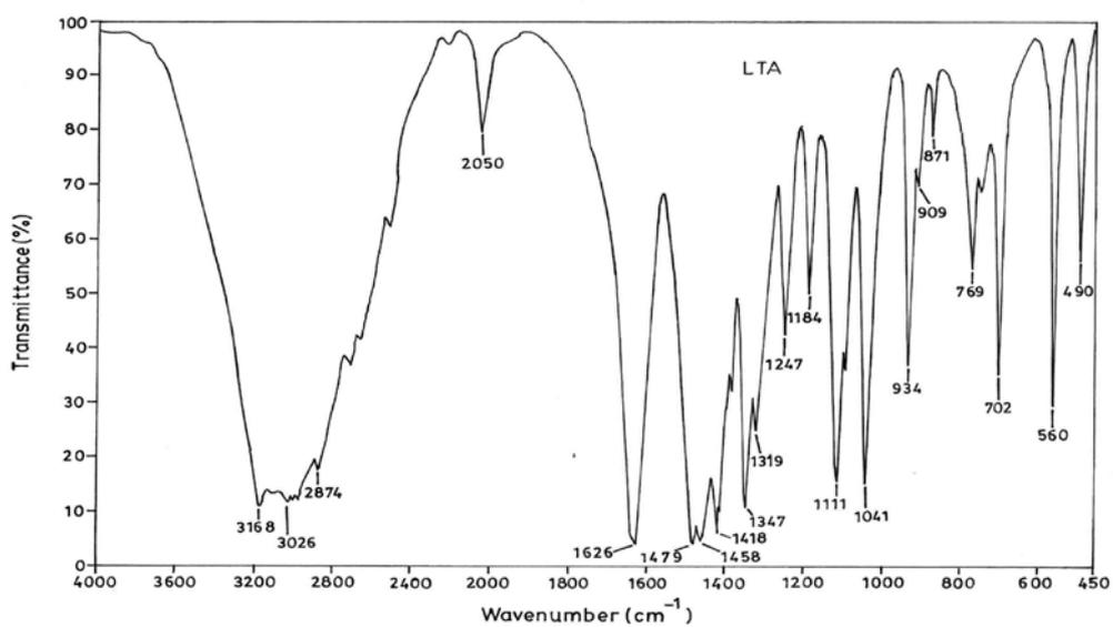
**Fig 5.3. FT-IR spectrum of LTA**
