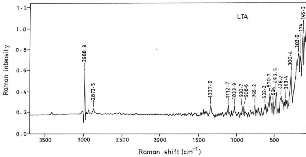
**Fig.5.4 FT- Raman spectrum of LTA**
