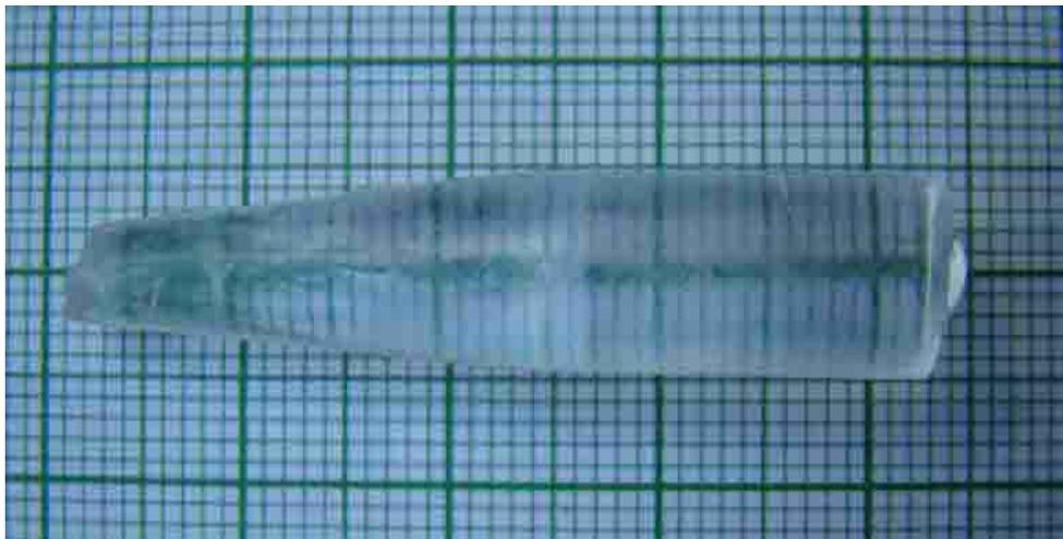
**Fig 5.1 LTA crystal grown by SR method**
