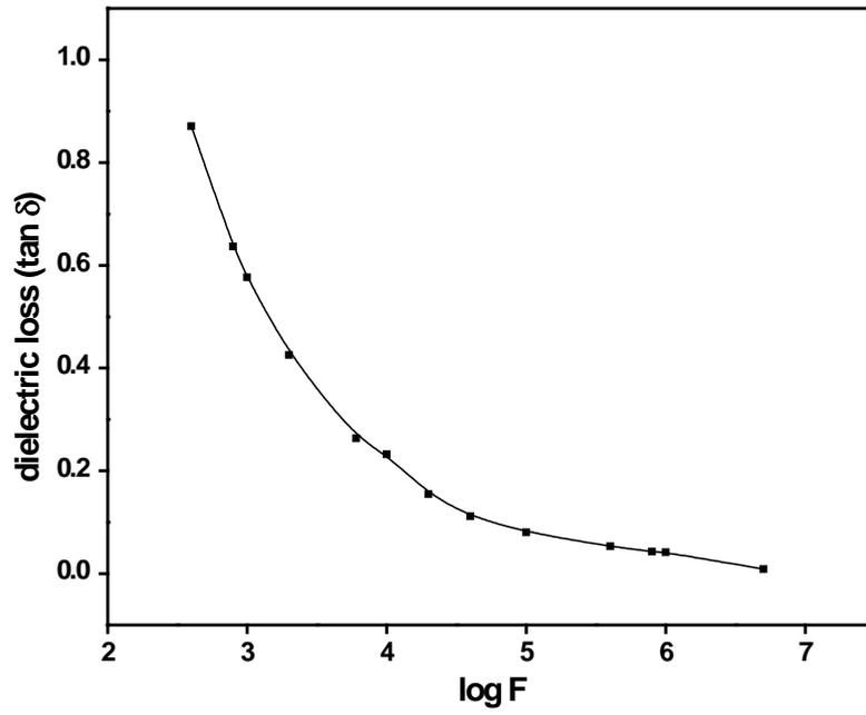
**Fig. 6.9** Plot of dielectric loss versus log frequency
