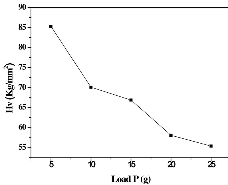
**Fig. 6.6 Vickers hardness profile of LAA**
