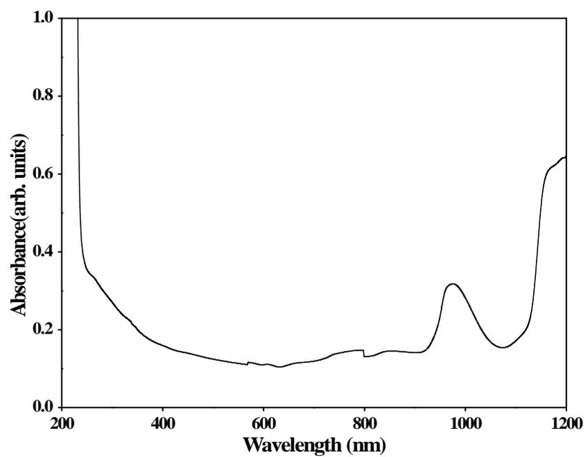
**Fig. 6.5 UV-Vis-NIR absorption spectrum of LAA crystal**
