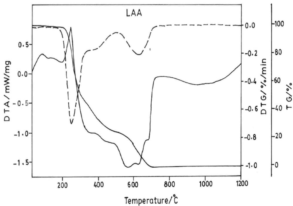
**Fig. 6.7 TGA and DTG thermogram of LAA crystal**
