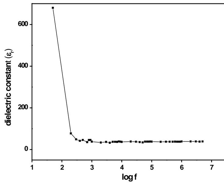
**Fig. 6.8 Plot of dielectric constant versus log frequency**
