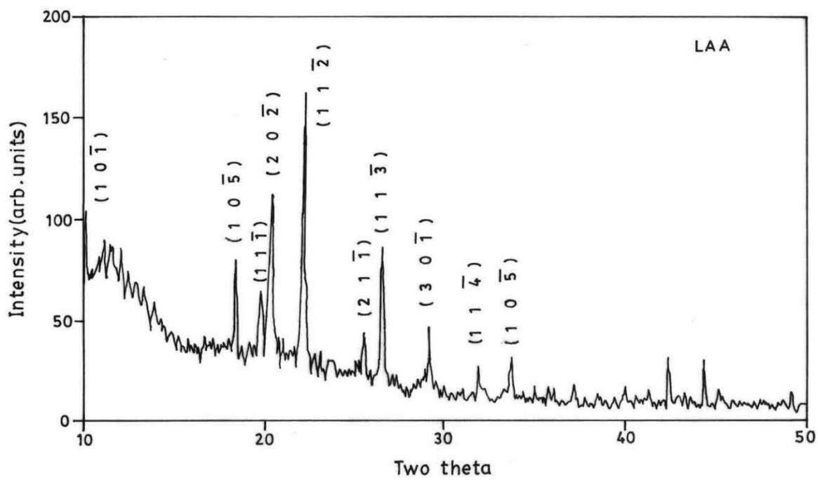
**Fig. 6.2. Powder XRD pattern of LAA crystal**
