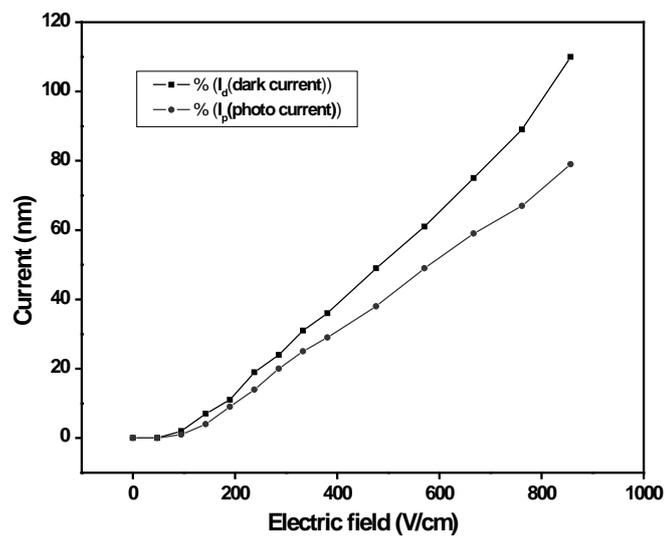
**Fig. 6.10** Field dependent conductivity of LAA single crystal
