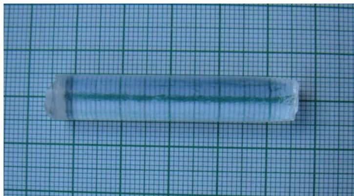
**Fig. 6.1. LAA crystal grown by SR method**
