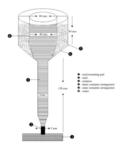
Fig 1.1 The schematic diagram of SR method apparatus
