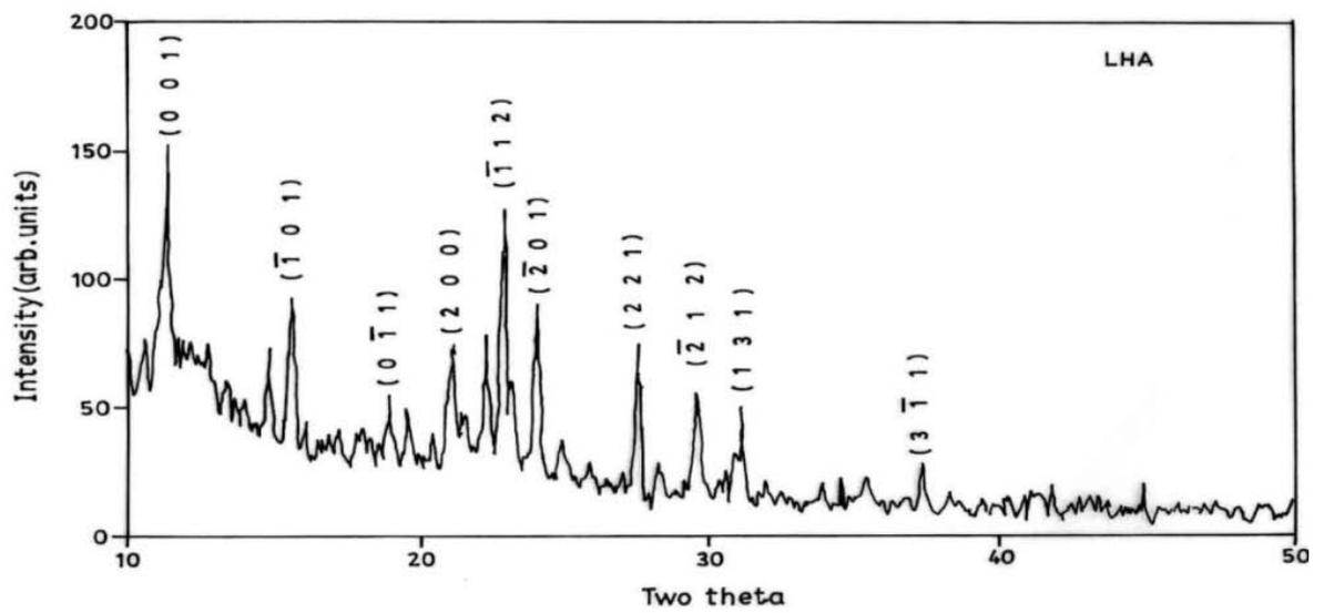
**Fig.3.2. Powder XRD pattern of LHA crystal**
