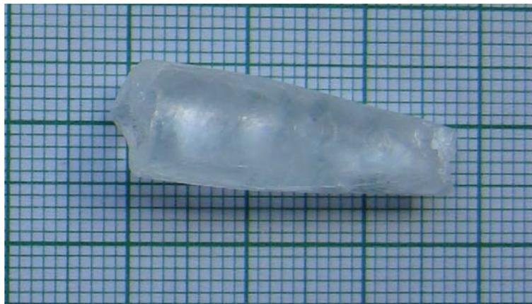
**Fig.3.1. LHA crystal grown by SR method**
