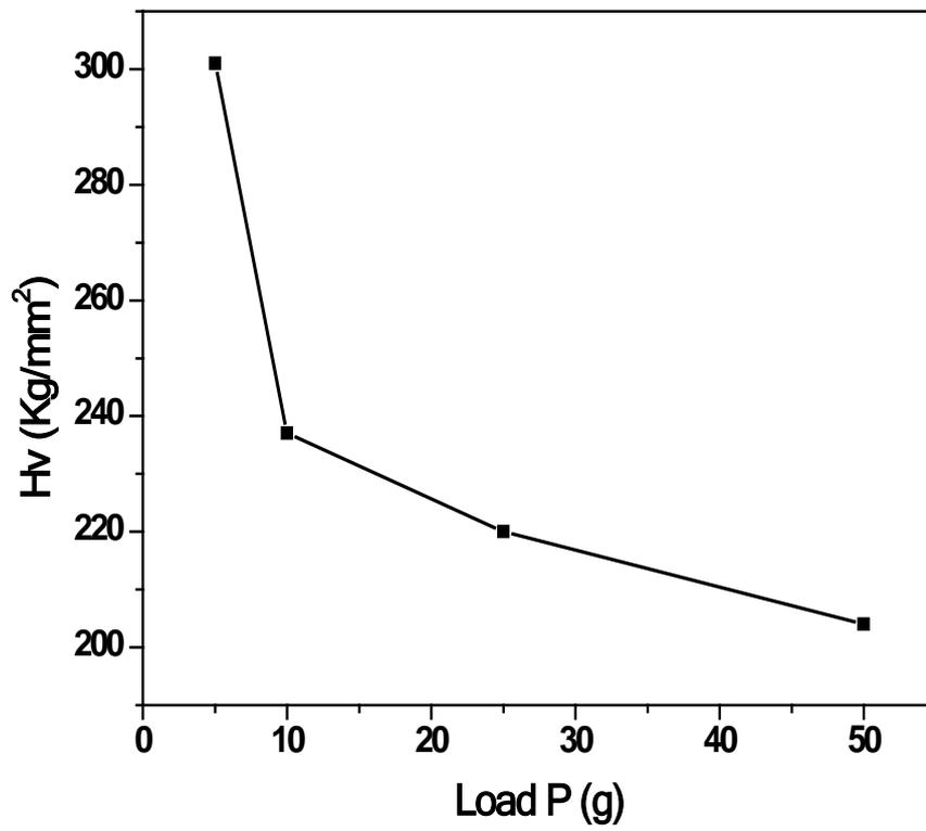
**Fig 3.6. Vickers hardness profile of LHA**
