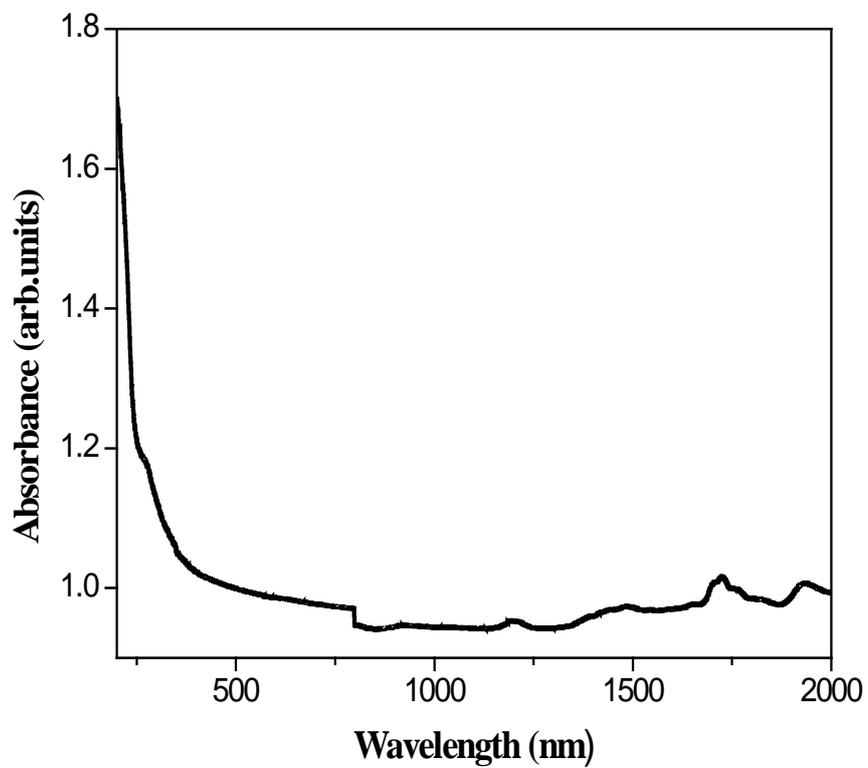
**Fig.3.5 UV-Vis-NIR absorption spectrum of LHA**
