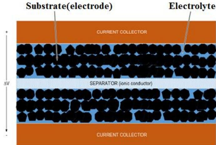
**Figure1.2:** Diagram of symmetric supercapacitor [4].
