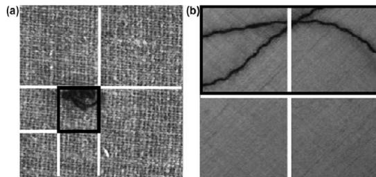
Figure- 2.2: Split scale image partitioning technique (a) multiple iterations of splitting at split scale 2 and (b) single iteration of splitting at split scale 2.
