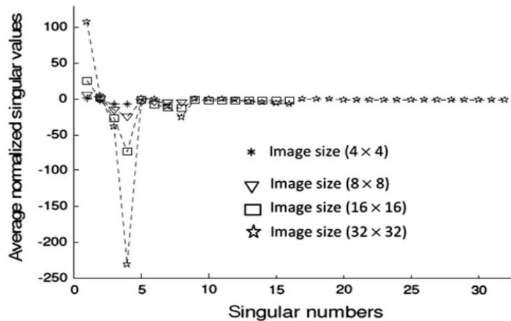
Figure-2.3(a): Plot of average normalized singular values for sub image size of  $(4 \times 4)$ ,  $(8 \times 8)$ ,  $(16 \times 16)$ ,  $(32 \times 32)$ .
