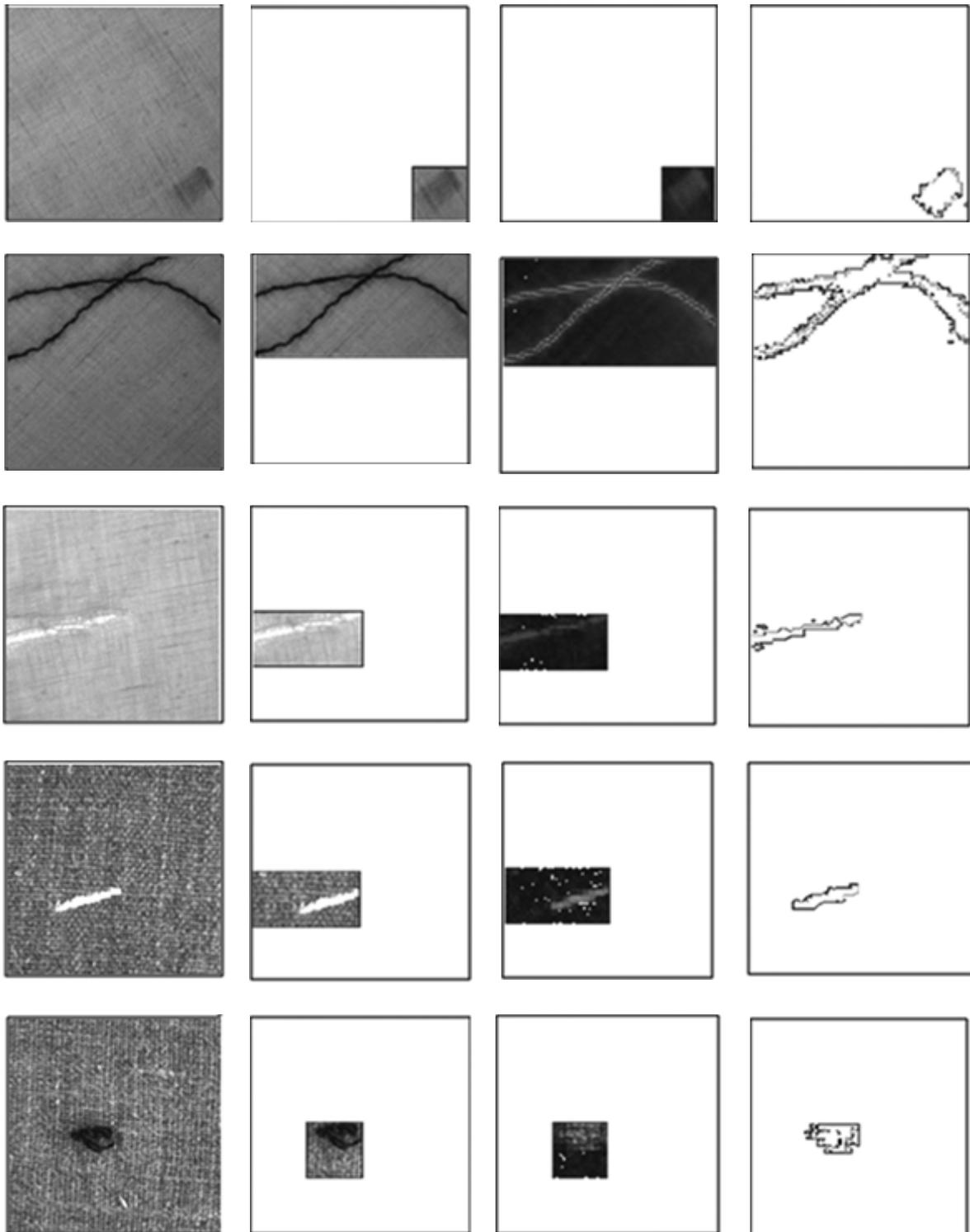
Figure-2.4: Images of test results; column 1: fabric image; column 2: partitioned image by split scale adaptive partitioning; column 3: images after SDV; column 4: images of defects after post-processing.
