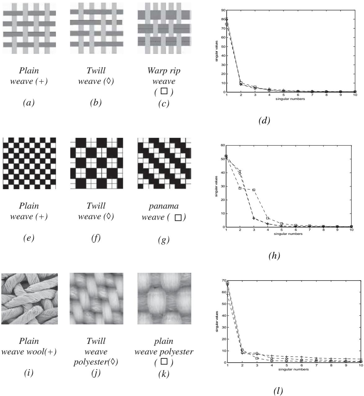
Figure-2.1: Synthetically generated fabric images (first and second rows) and actual fabric images (third row) and their SVD plots up to 10 singular numbers (fourth column).
