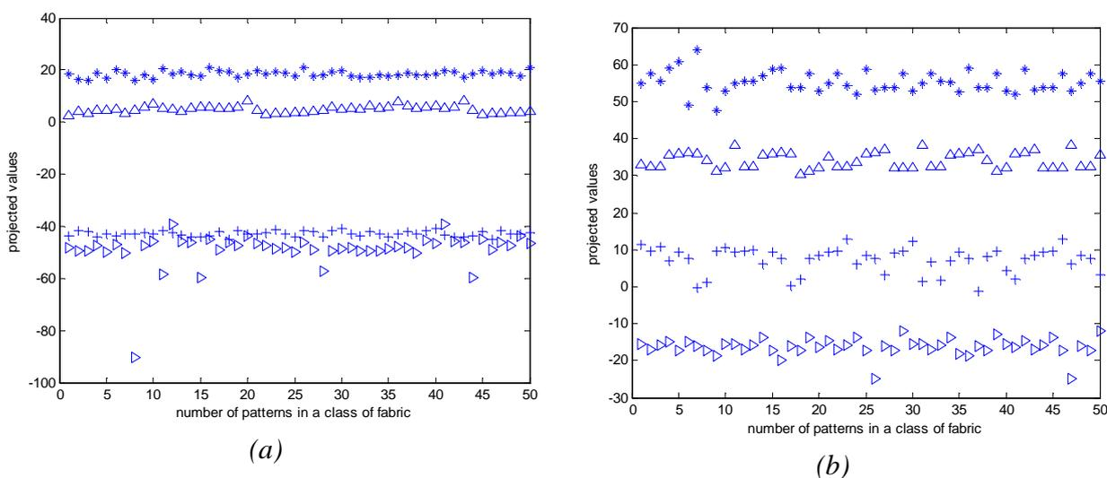
Figure- 4.3: plot of optimum projected values of test fabric samples of all fabric classes (a) in non optimized Haralick space, (b) in optimized Haralick space. Different symbols indicate different fabric classes.
