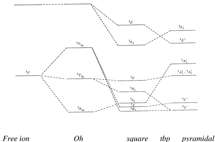
**Fig 2.4** Energy level scheme for triplet states in five coordinated Ni(II)
