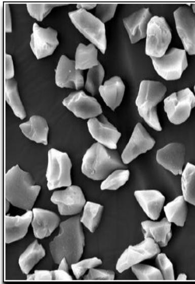
**Fig. 1.11** Column packed with irregular particles that lack mechanical strength:
