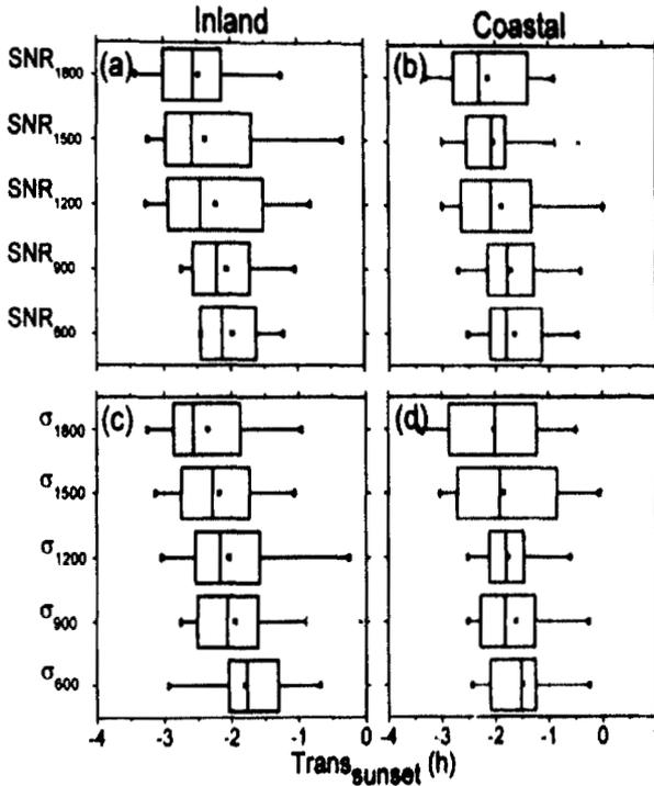
Figure 6.6: Top-to-bottom evolution of start time of AT with reference to the time of sunset, obtained from profiler-derived SNR (a & b) and  $\sigma$  (c & d) at an inland (left panels) and a coastal station (right panels), respectively.
