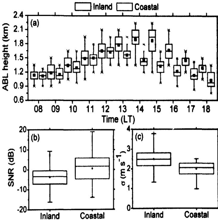
Figure 6.3: Temporal variation of the distribution of (a) mean ABL height at inland (blue) and coastal (red) station. Boxplots of (b) SNR (c)  $\sigma$  during the afternoon period (11-13 LT) below 1.5 km. The mean is taken over 53 (69) inland (coastal) days.
