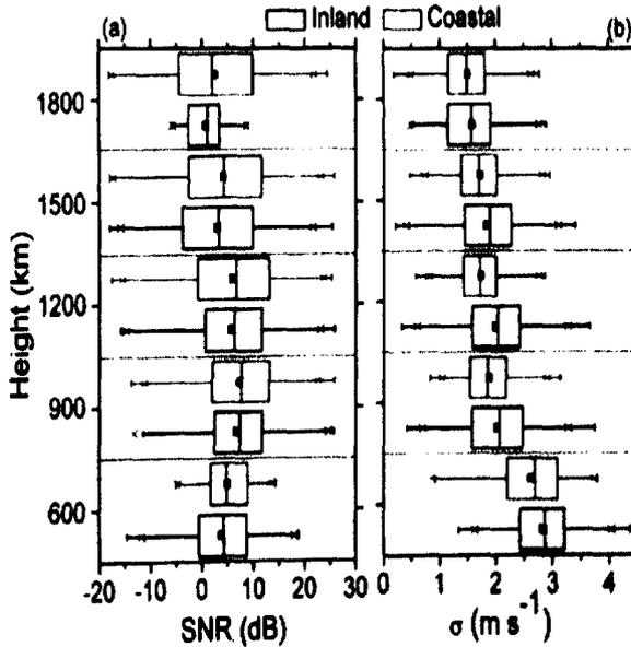
Figure 6.8: Vertical variation of distributions of SNR (left panel) and  $\sigma$  (right panel) obtained during the PST period between inland and coastal stations.
