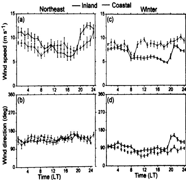
Figure 6.4: Temporal variation of mean low-level winds (below 1.5 km) obtained by WPRs (a & c) wind speed (b & d) wind direction. The mean is taken over 27 (26) and 30 (30) days for northeast (winter) seasons at inland and coastal station, respectively.
