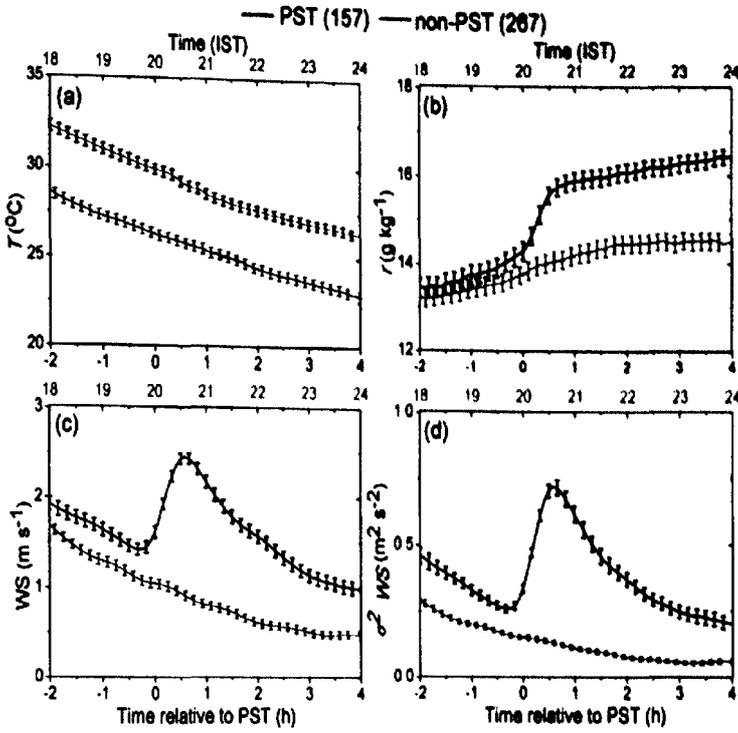
Figure 5.7: Temporal variation of mean surface state parameters (a)  $T$ , (b)  $r$ , (c)  $WS$  and (d)  $\sigma^2 ws$  during PST night (bottom axis) and non-PST night (top axis).
