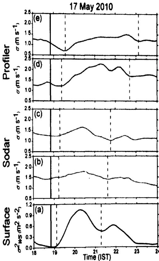
Figure 5.2: Temporal variation of MBLM-derived (a)  $\sigma_{ws}^2$ , (b-c) sodar-derived  $\sigma$  and (d-e) profiler-derived  $\sigma$ . The sodar- and profiler- $\sigma$  are plotted at two representative levels each (300 and 450 m for sodar and 900 and 1500 m for profiler). Vertical black solid line indicates the time of sunset and vertical dashed green (cyan) lines indicate the start (end) time of PST.
