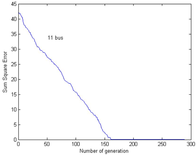
Fig. 5.6: Variations of the sum square error with the generations for 11 bus test system for two-stage GA based load flow with 10-population size
