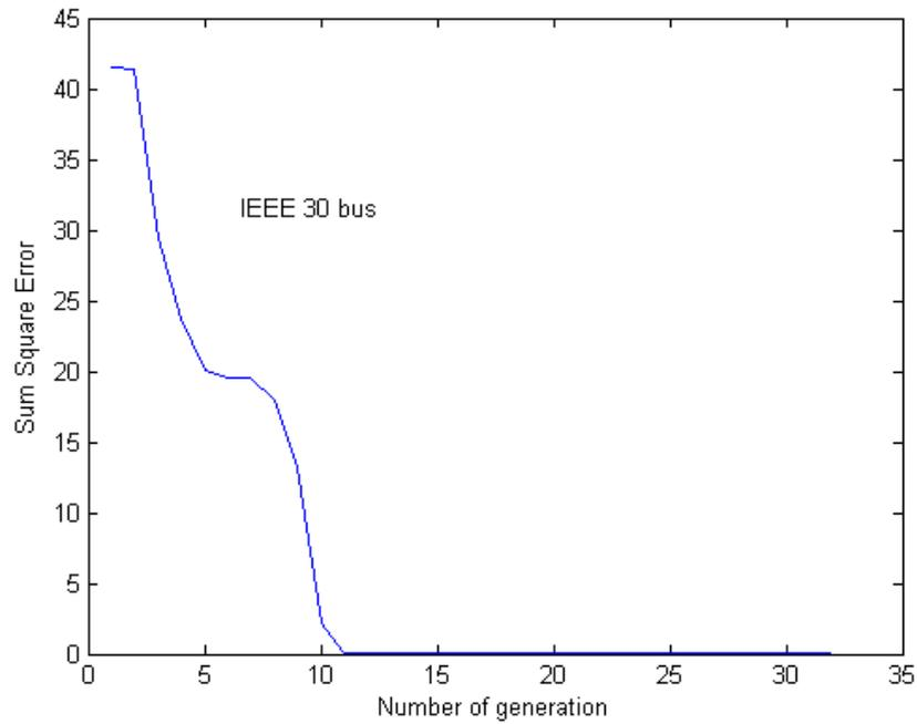
Fig. 5.16: Variations of the sum square error with the generations for IEEE 30 bus test system for the two-stage GA based load flow with linear perturbation for the population size of 10
