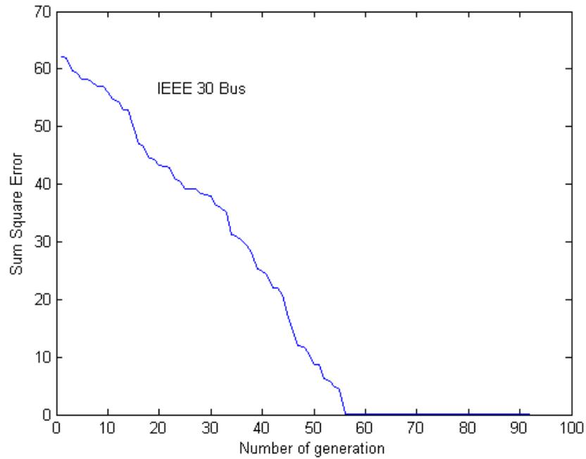
Fig. 5.12: Convergence characteristic of IEEE 30 bus test system with 10-population size for the two-stage GA with local search
