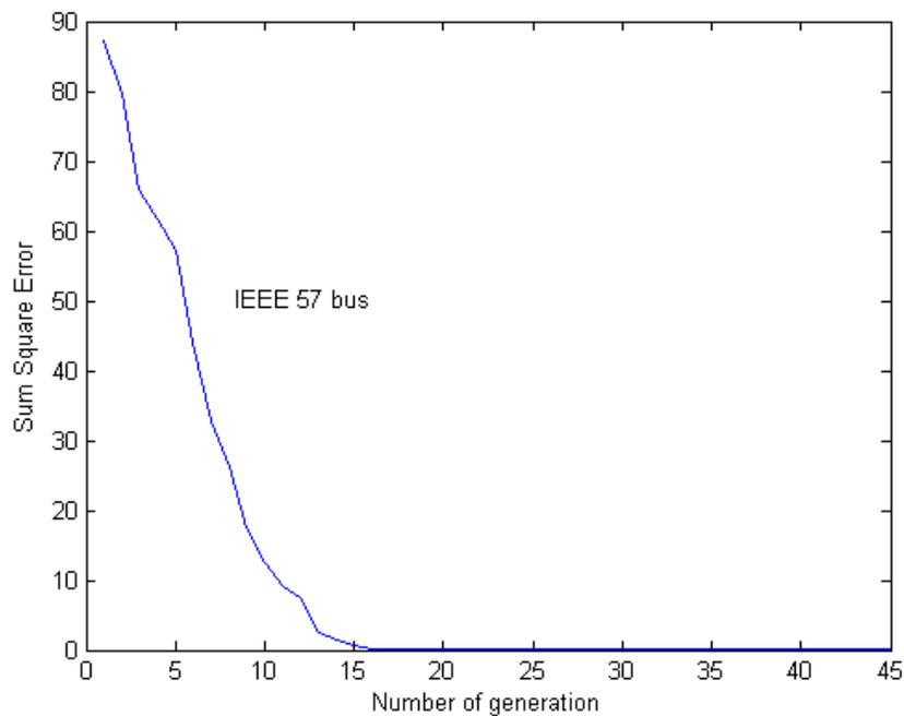
Fig. 5.17: Variations of the sum square error with the generations for IEEE 57 bus test system for the two-stage GA based load flow with linear perturbation for the population size of 10
