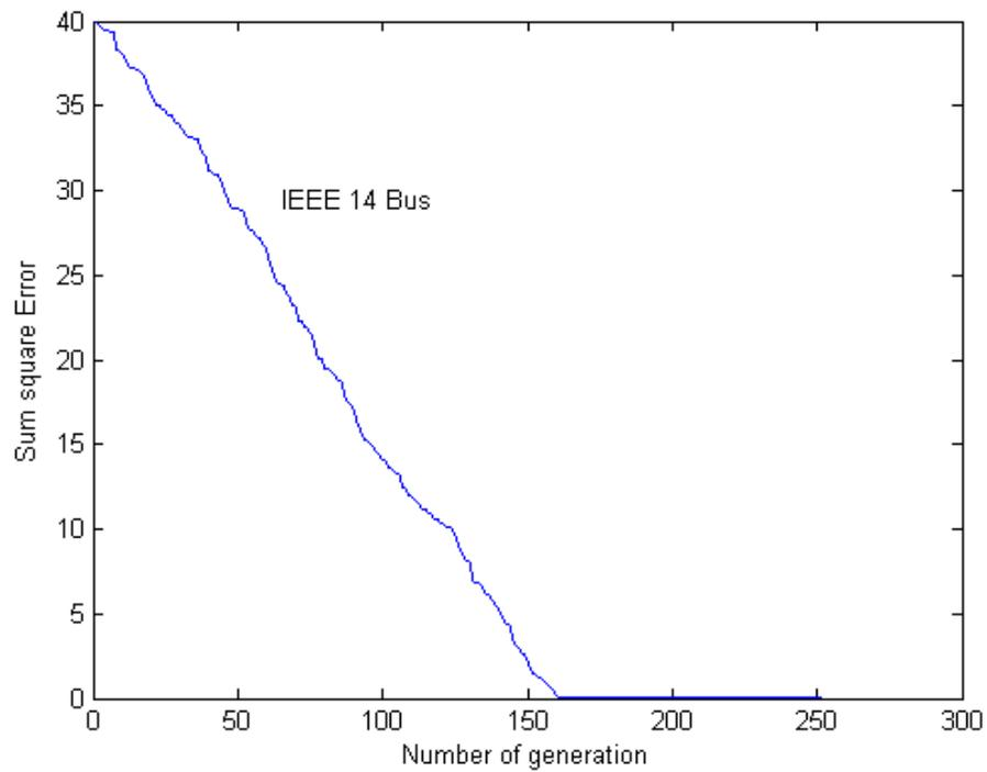
Fig. 5.7: Variations of the sum square error with the generations for IEEE 14 bus test system for two-stage GA based load flow with 10-population size
