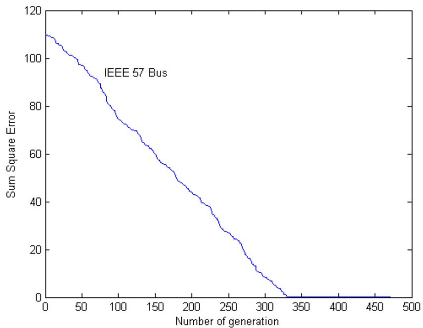
Fig. 5.9: Variations of the sum square error with the generations for IEEE 57 bus test system for two-stage GA based load flow with 10-population size
