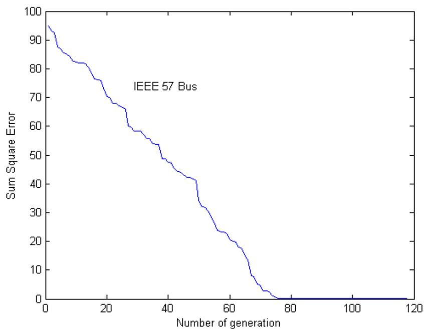
Fig. 5.13: Convergence characteristic of IEEE 57 bus test system with 10-population size for the two-stage GA with local search
