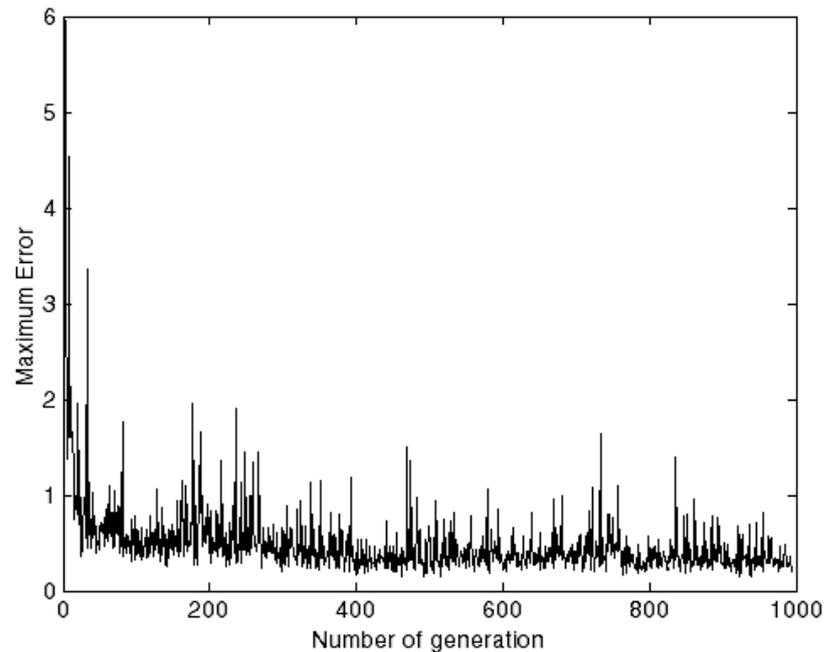
Fig. 5.1: Convergence characteristics of simple GA based power flow for IEEE 30 bus test system with 500-population size
