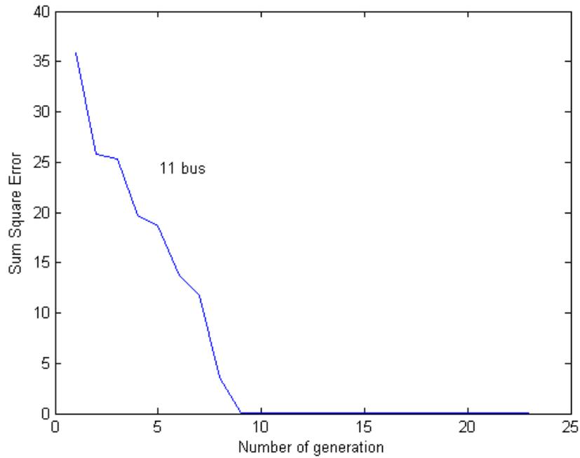
Fig. 5.14: Variations of the sum square error with the generations for 11 bus test system for the two-stage GA based load flow with linear perturbation for the population size of 10
