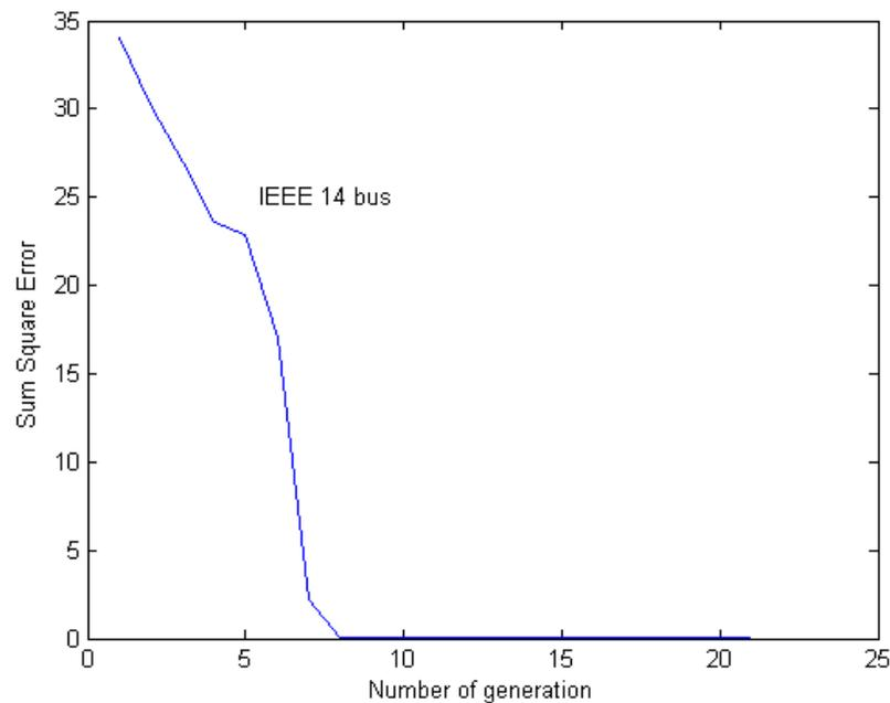
Fig. 5.15: Variations of the sum square error with the generations for IEEE 14 bus test system for the two-stage GA based load flow with linear perturbation for the population size of 10
