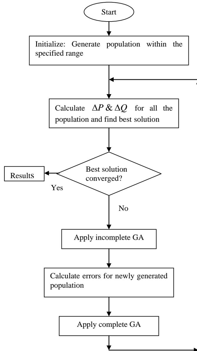
Fig. 5.5: Flowchart of the two-stage GA based load flow
