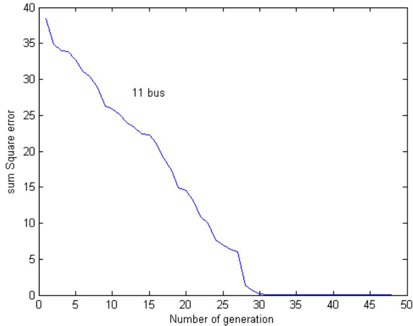
Fig. 5.10: Convergence characteristic of 11-bus test system with 10-population size for the two-stage GA with local search
