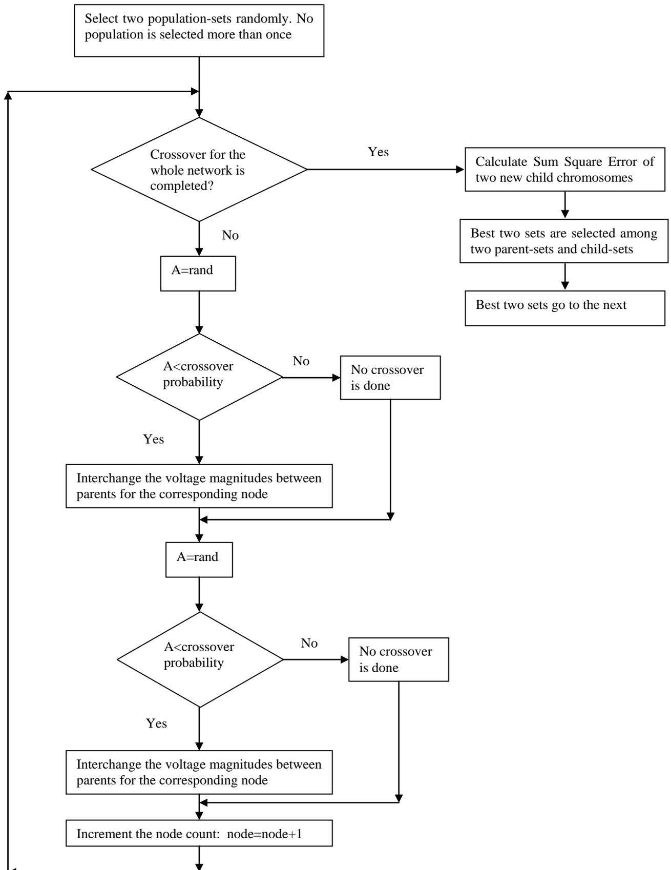
Fig.5.3. Flowchart of the crossover operation used in the complete GA stage
