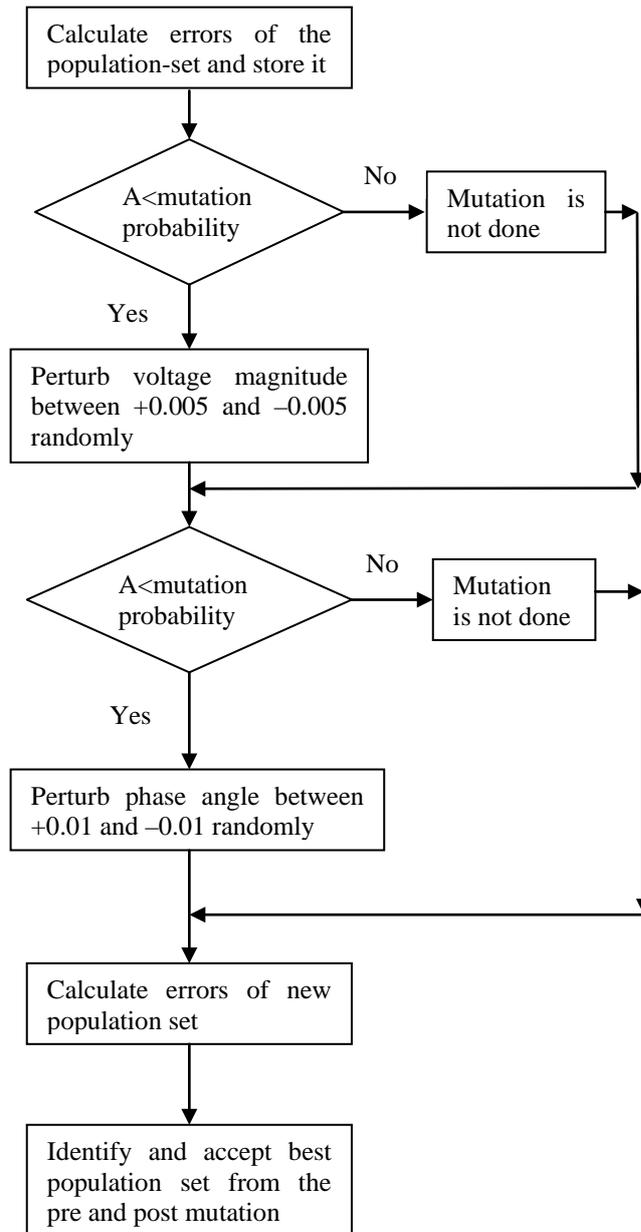
Fig. 5.4: Flowchart of the mutation operation used in the complete GA stage
