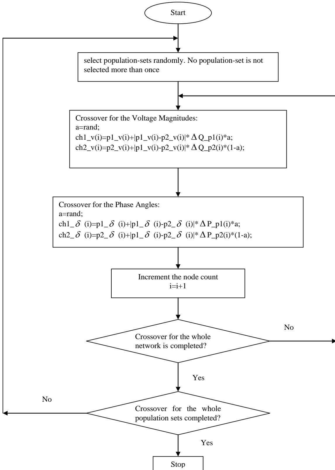
Fig.5.2. Flowchart of the crossover operation used in the incomplete GA stage
