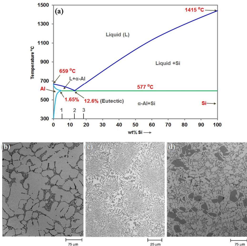
**Figure 1.6 Metallurgical Features of Al-Si Alloy (Warmuzek 2004)**
