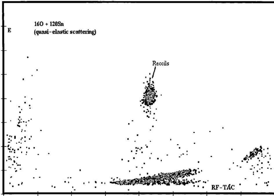
Figure 5.2: A two dimensional plot of TOF vs Energy for the quasi-elastic scattering for  $^{16}\text{O} + ^{120}\text{Sn}$ . The recoiling target like particles are clearly separated from the the background.
