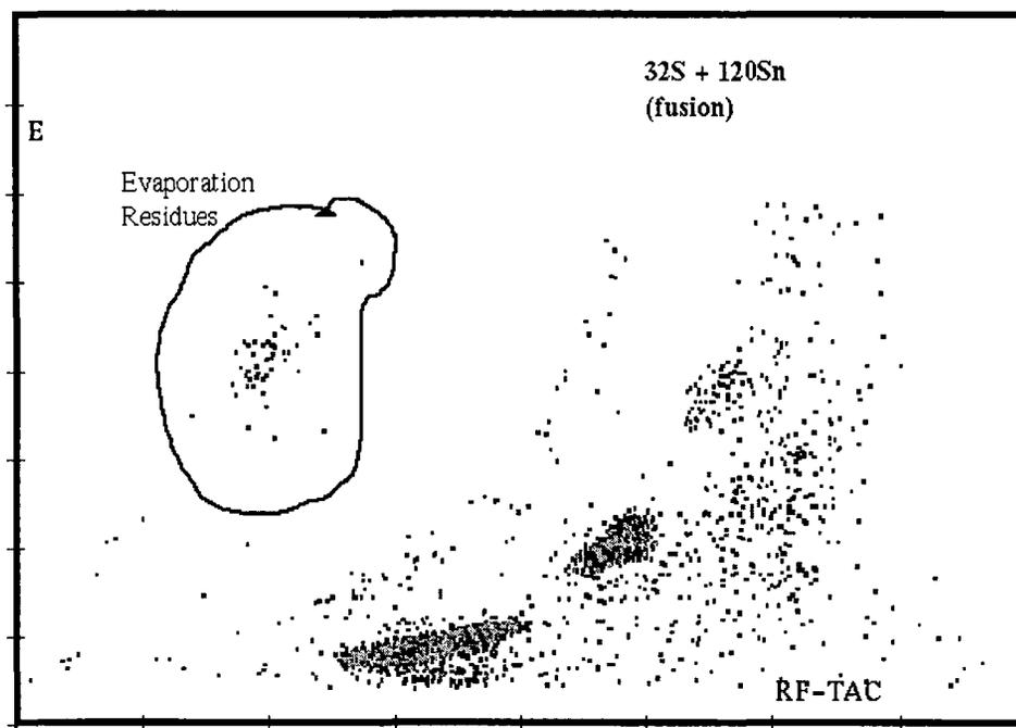
Figure 5.1: A typical two dimensional plot of TOF vs Energy at a very sub-barrier energy. A clear separation of the ER's from the background can be seen.
