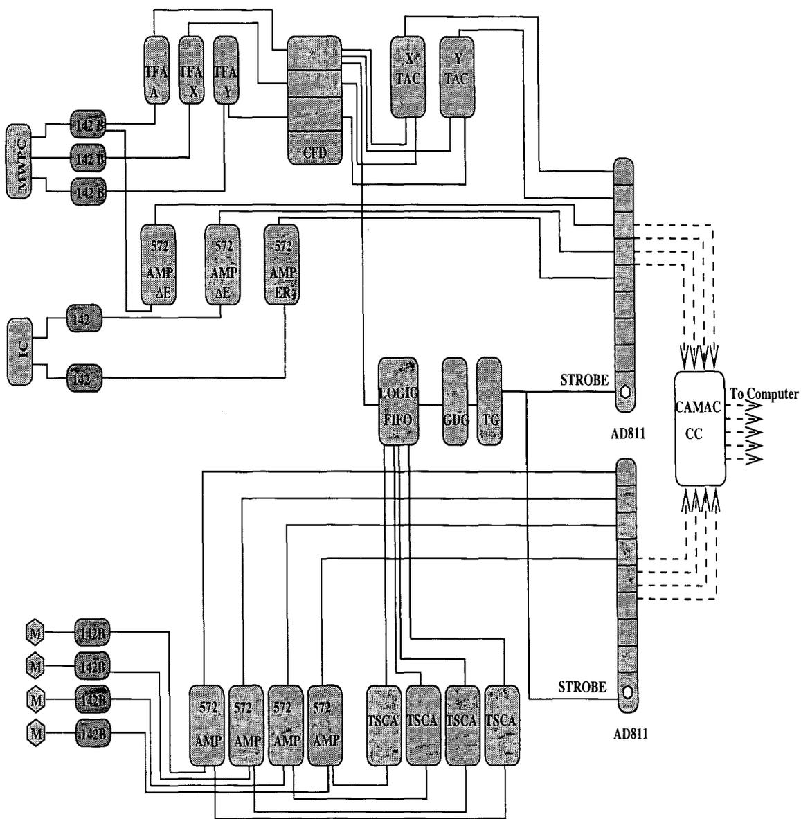
Figure 5.4: Block diagram of the electronic setup for the experiments.
