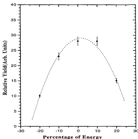
Figure 5.6: Measured energy acceptance of HIRA using  $\alpha$  source.
