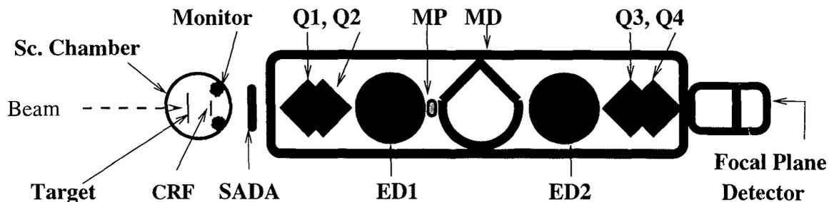
**ED1, ED2 - Electric Dipoles ; MD - Magnetic Dipole ;
