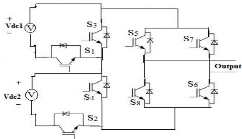
**Figure 3.4 Asymmetrical Seven level Cascaded H bridge multi-level inverter using Sub Multi-level inverter**
