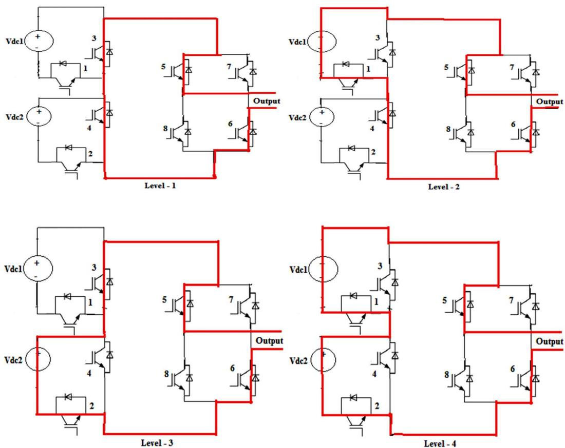
**Figure 3.5 Levels of Operation of proposed seven-level asymmetrical multi-level inverter Switching Pattern**
