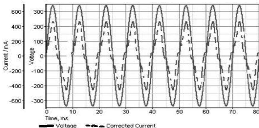
**Figure 3.9 Power Factor at the supply of proposed converter**
