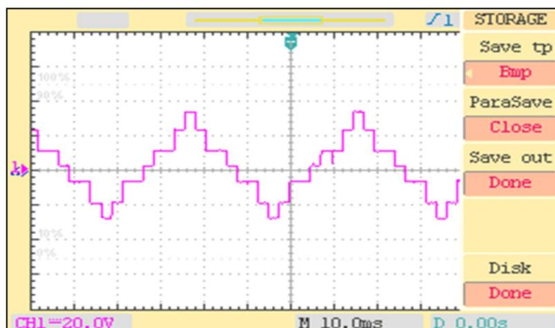
**Figure 3.17 Inverter output voltage (scale 300V/div), Time scale (5ms/div)**
