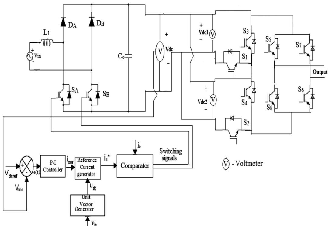
**Figure 3.2 Circuit diagram of the Closed loop controlled Bridgeless PFC Boost converter fed inverter**
