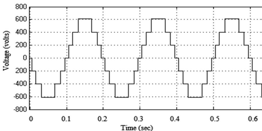
**Figure 3.11 Seven-level inverter output voltage waveform**
