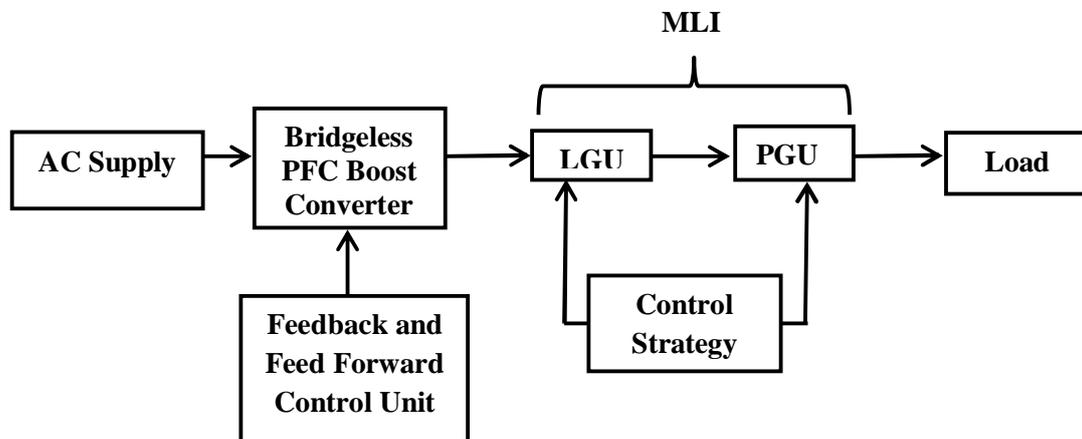
**Figure 3.1 Block diagram of proposed converter fed inverter**
