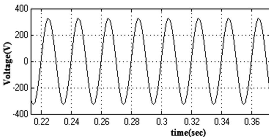
**Figure 3.7 Input Voltage waveform of the converter**
