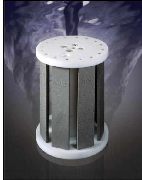
**Figure 9. (b) Samples mounted between PTFE disks**
