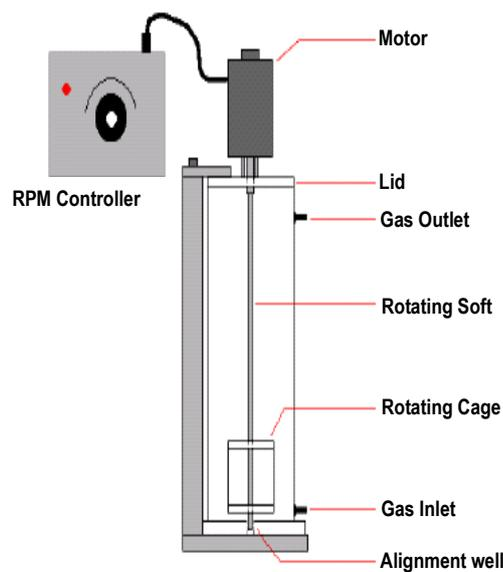
**Figure 7. Schematic diagram of the rotating cage**
