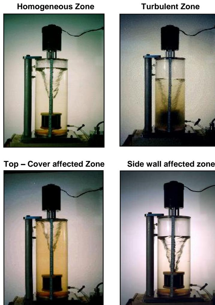
**Figure 8. Flow patterns in rotating cage**
