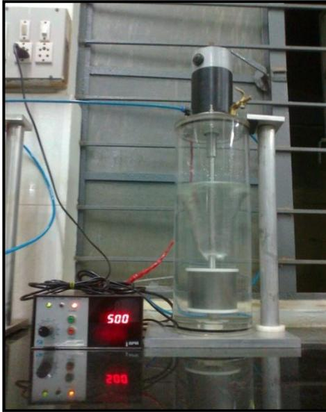
**Figure 9. (a) Rotating cage at constant 500rpm**
