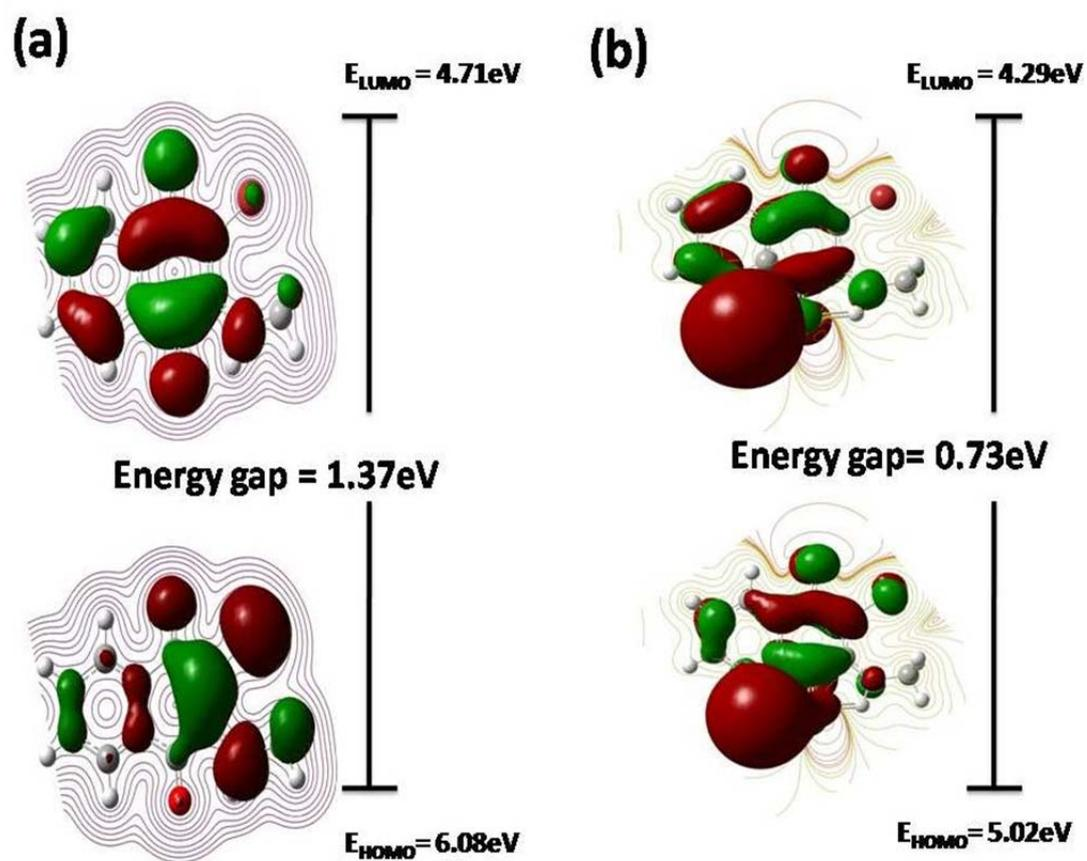
**Figure 5.1** HOMO and LUMO plot of (a) BMANQ molecule and (b) BMANQ molecule on Ag NPs.
