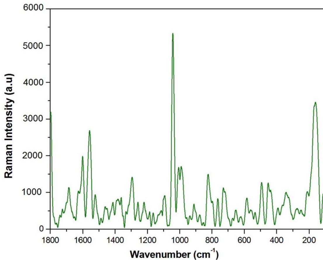
**Figure 5.4** Surface Enhanced Raman spectrums (SERS) of BMANQ molecule on AgNPs.
