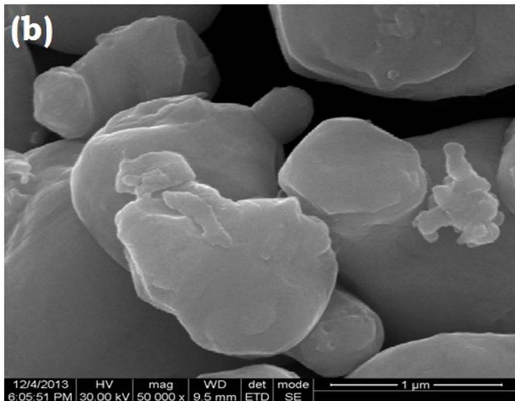
**Figure 3.4** FESEM images of prepared Ag NPs.
