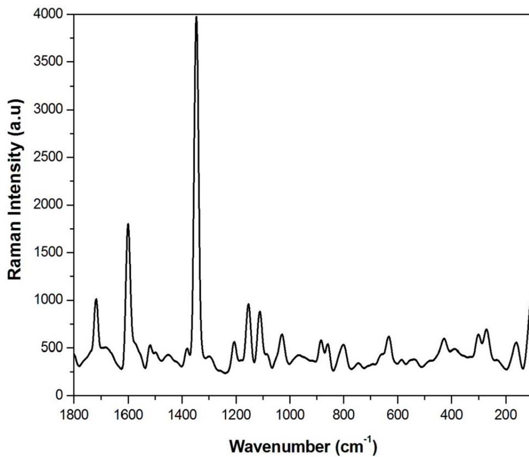
**Figure 3.7** Normal Raman spectrums (nRs) of CNPSA molecule.
