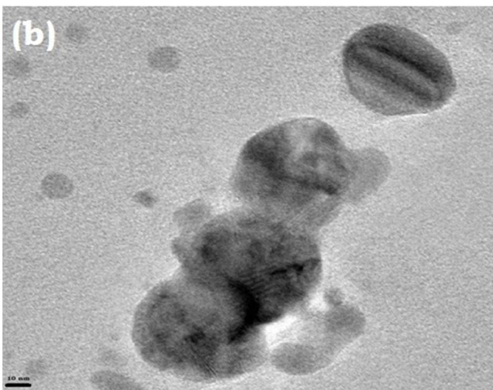
**Figure 3.3** HR-TEM images of prepared Ag NPs in different magnifications.
