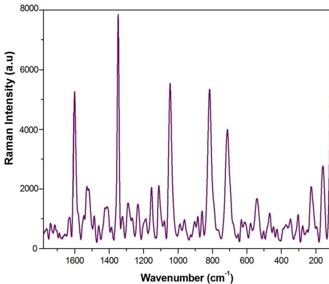
**Figure 3.8** Surface Enhanced Raman Spectrums (SERS) of CNPSA molecule on Ag NPs.
