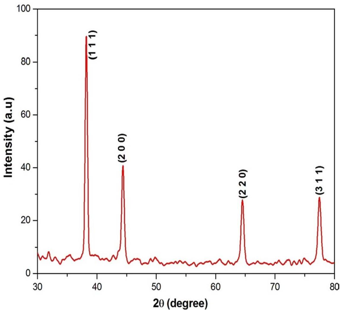
**Figure 3.1** X-Ray diffraction pattern of prepared Ag NPs.
