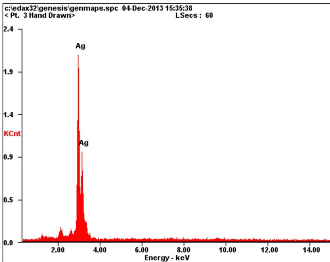
**Figure 3.5** Energy Dispersion Spectrum (EDS) of prepared AgNPs.
