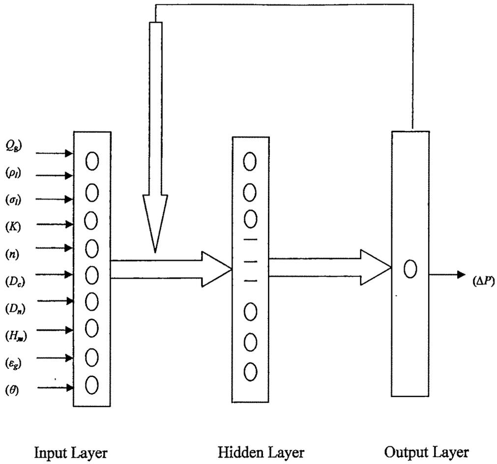
Fig. 4.3 Schematic diagram of neural network for pressure drop
