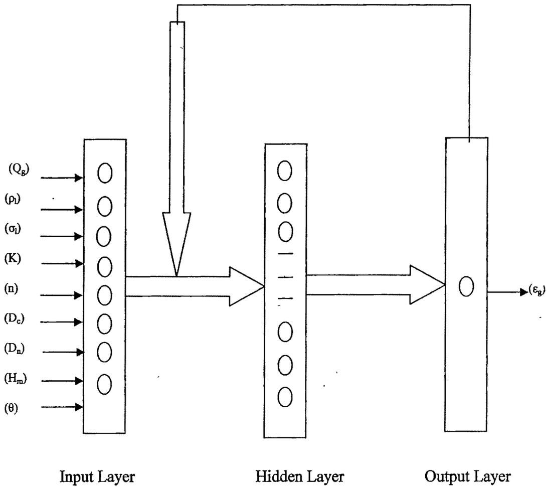
Fig. 4.2 Schematic diagram of neural network for gas holdup
