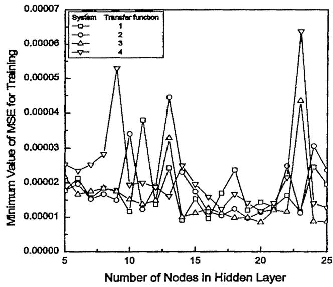
Fig. 4.4 Variation the minimum value of MSE with the number of nodes in a hidden layer for four different transfer functions for gas holdup
