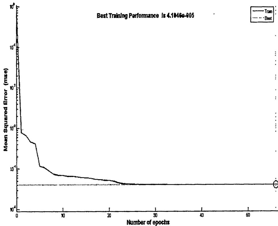
Fig. 4.9 Variation of the average MSE for training over 20 different runs vs the number of epochs for transfer functions 4 in the hidden layer for pressure drop
