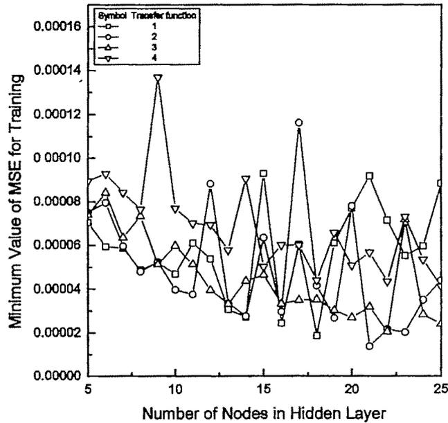
Fig. 4.5 Variation the minimum value of MSE with the number of nodes in a hidden layer for four different transfer functions for pressure drop
