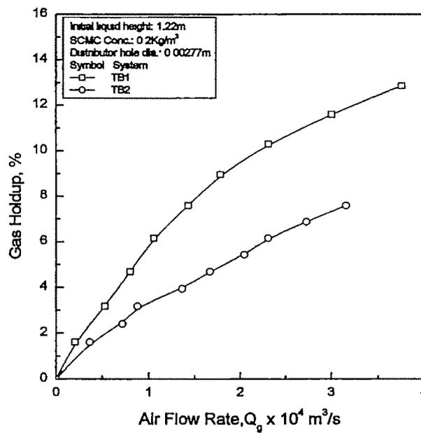
Fig. 3.9 Effect of the taper angle on holdup
