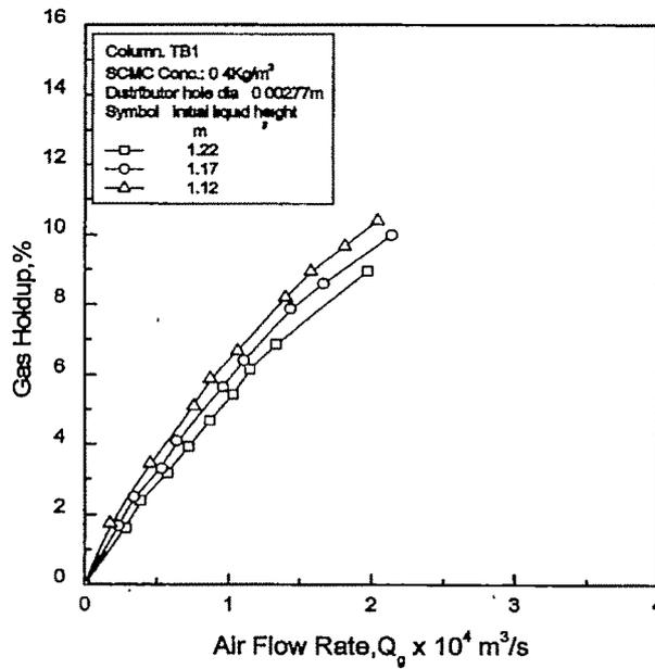
Fig. 3.3 Variation of gas holdup with gas flow rate at different clear liquid height
