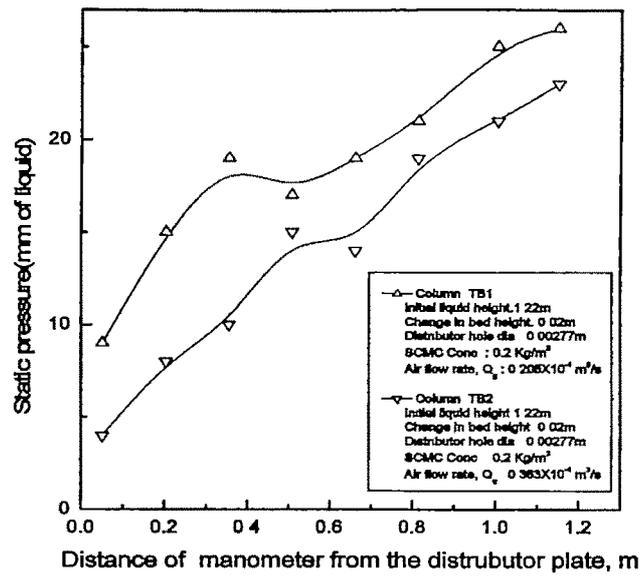
Fig. 3.2 Variation of static pressure with distance of manometer from the distributor Plate
