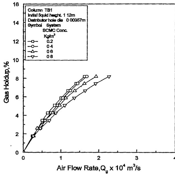
Fig. 3.4 Variation of gas holdup with gas flow rate at different SCMC solution concentration
