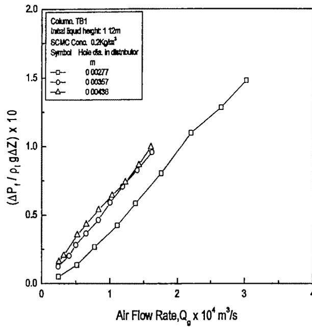
Fig. 3.8 Variation of frictional pressure drop with gas flow rate at different hole diameter of the gas distributor
