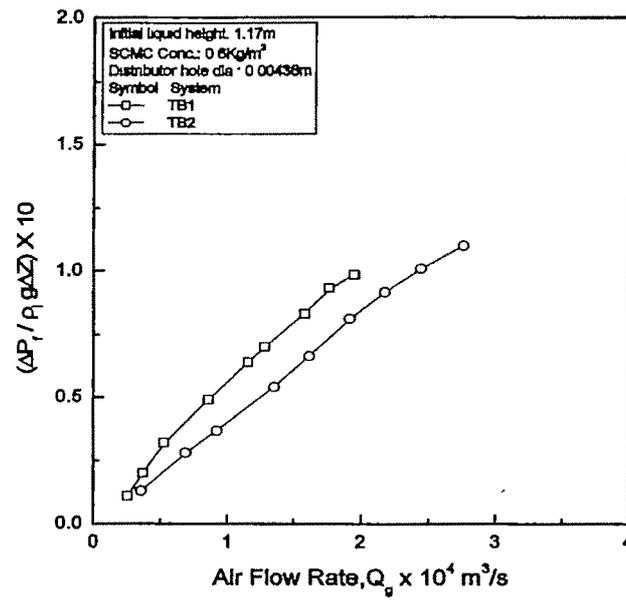
Fig. 3.10 Effect of the tapered angle on frictional pressure drop
