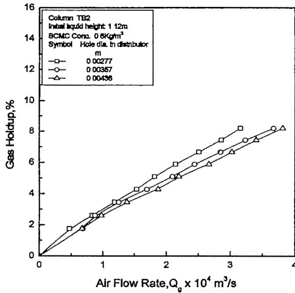
Fig. 3.7 Variation of gas holdup with gas flow rate at different hole diameter of the gas distributor
