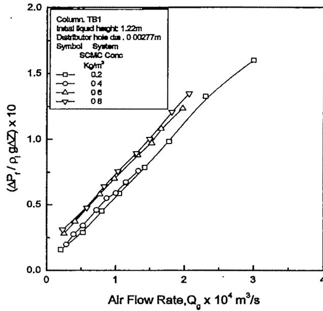
Fig. 3.6 Variation of frictional pressure drop with gas flow rate at different SCMC solution concentration
