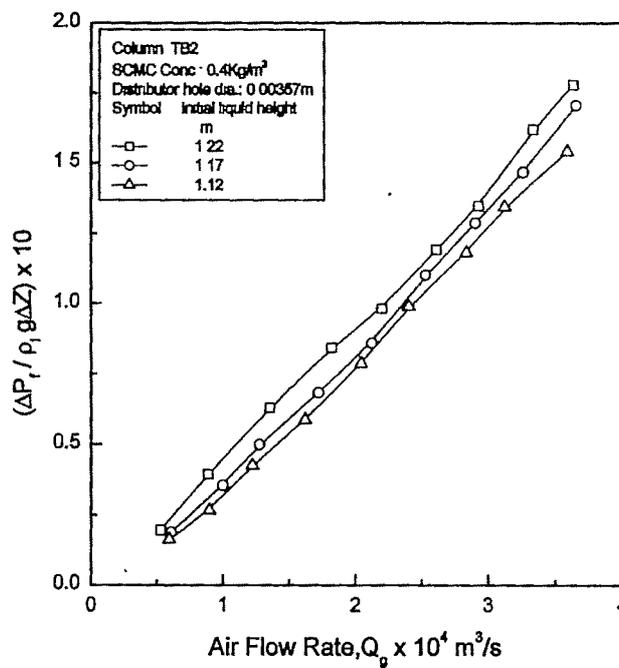
Fig. 3.5 Variation of frictional pressure drop with gas flow at different clear liquid height
