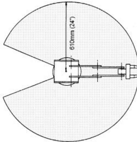
**Figure 1.6 Operating Range (Top View)**
