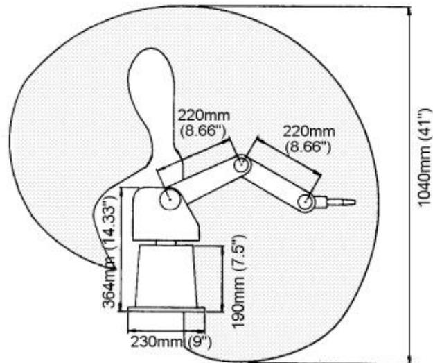
**Figure 1.7 Operating Range (Side View)**
