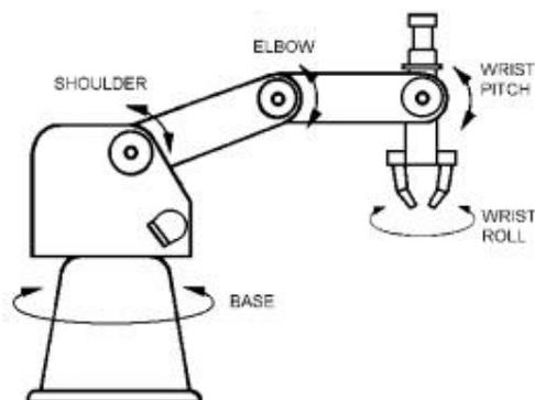
**Figure 1.3 SCORBOT arm Joints**
