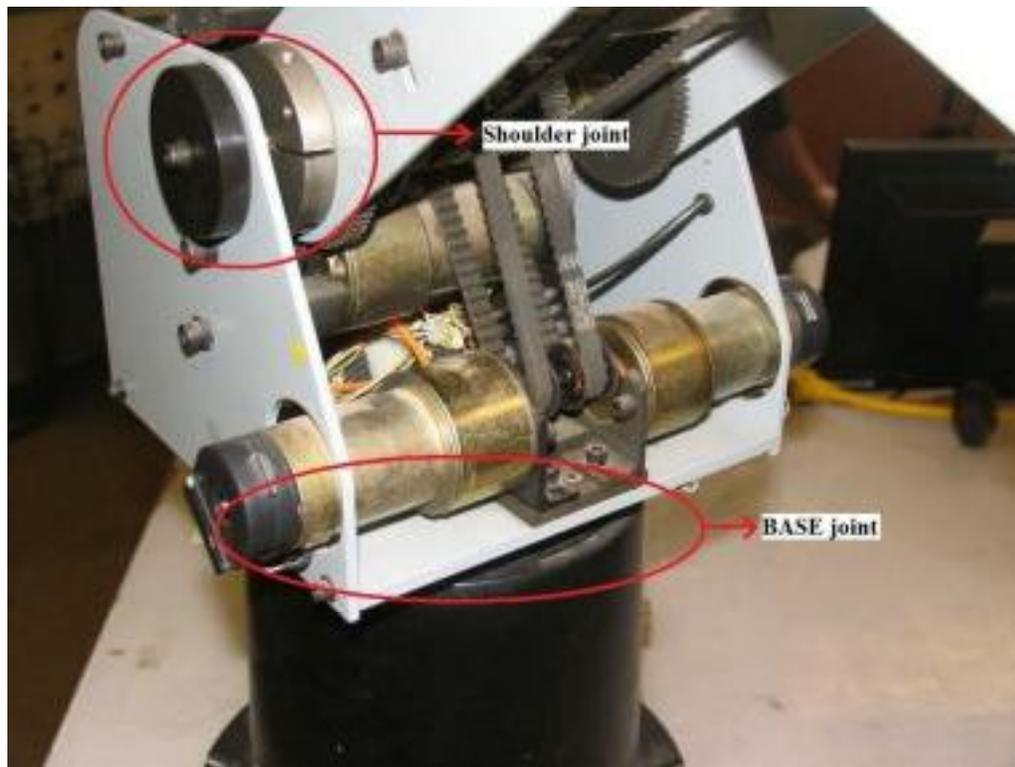
**Figure 1.4 SCORBOT base and shoulder Joints**
