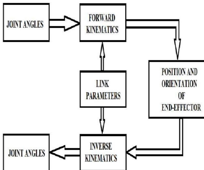
**Figure 1.1 Forward and Inverse Kinematics**
