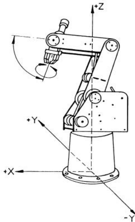
**Figure 1.11 SCORBOT XYZ Coordinate System**
