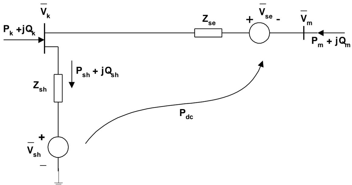
Fig. 2.4 Two voltage source equivalent circuit of UPFC
