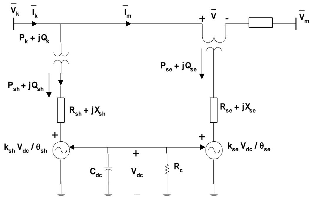
**Fig.2.5 The UPFC model used in the Present Work**
