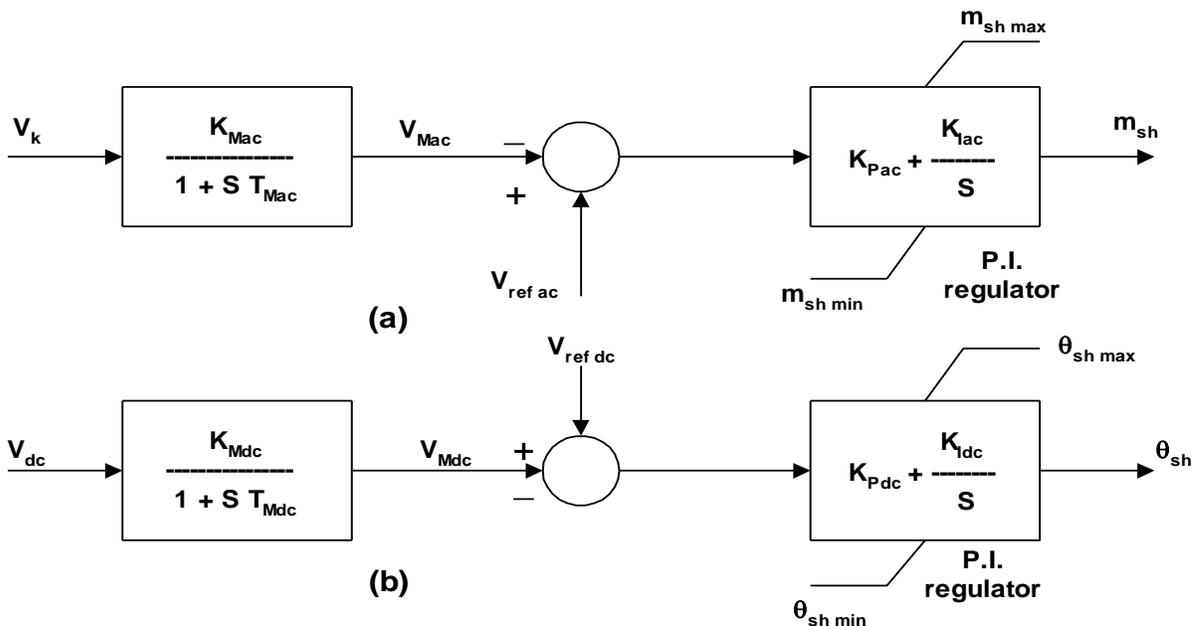
Fig. 2.6 UPFC shunt control block diagrams
