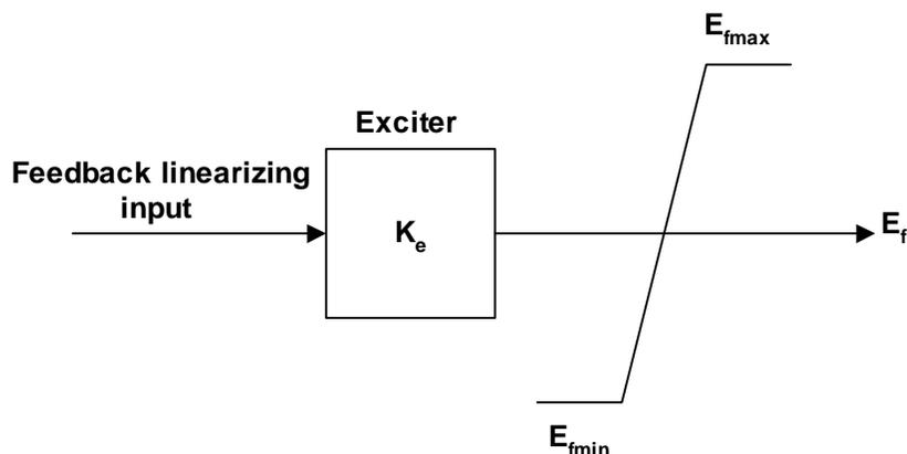
Fig.2.2: Excitation system as used in the present work
