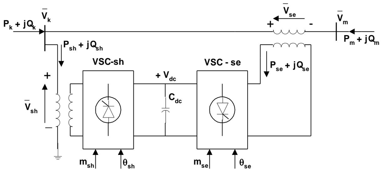
Fig. 2.3 Schematic diagram of UPFC
