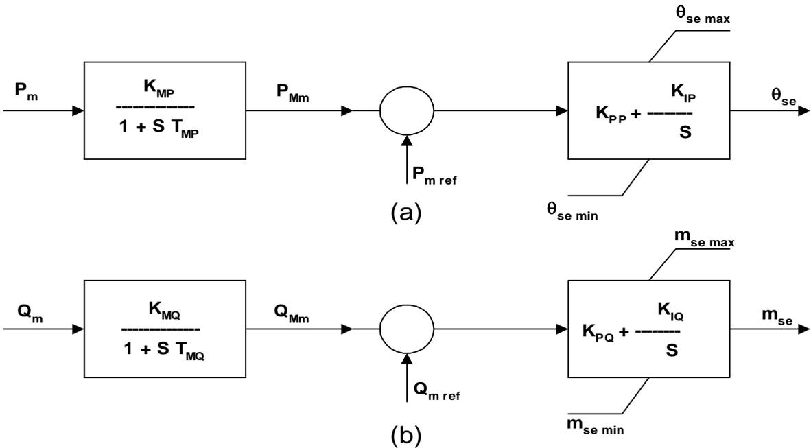
Fig.2.7 UPFC Series control block diagrams
