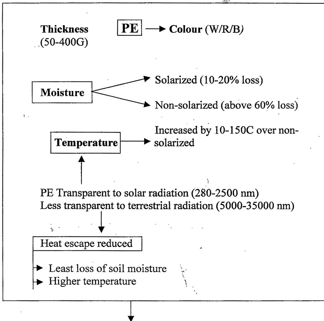
**Fig.19 : Effect on soil moisture and temperature**
