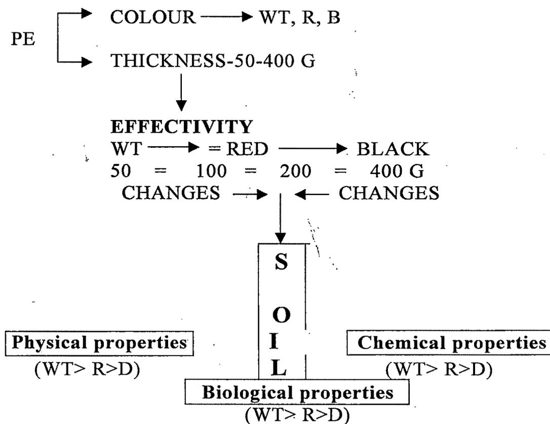
**Fig.18 : Effect of soil solarization on soil properties**
