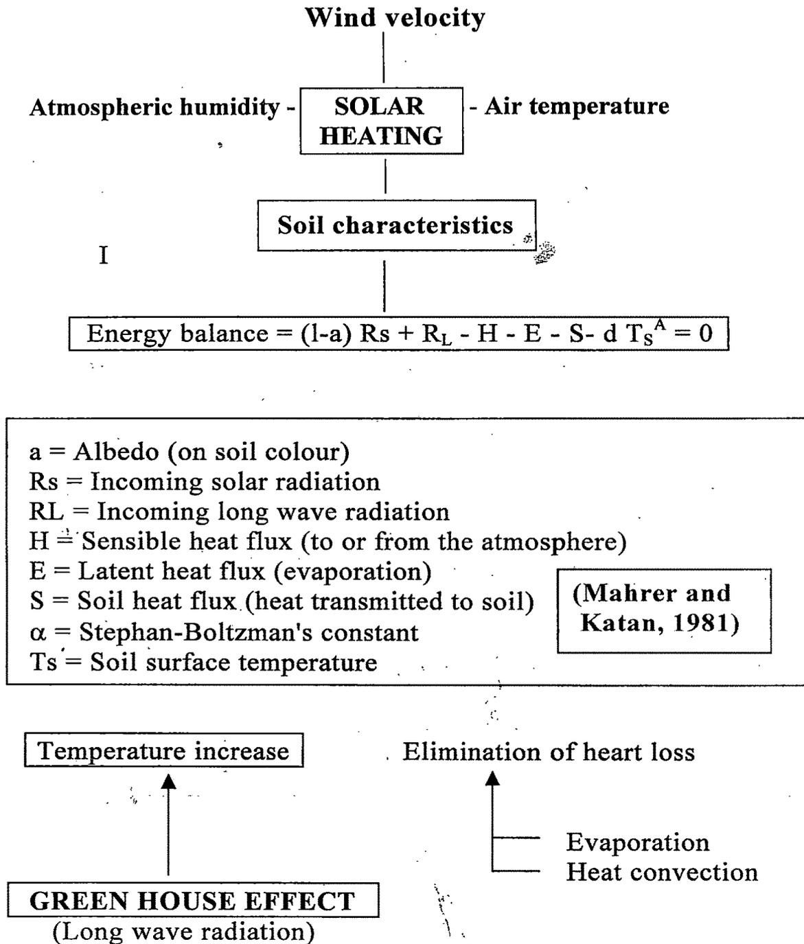
**Fig.20 : Calculation of temperature in soil**
