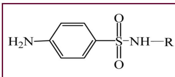
Figure 1.2 Structural formula of sulfonamide
