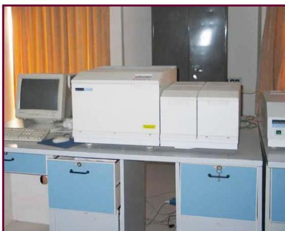
**Figure 2.11 Infrared Spectrophotometer**
