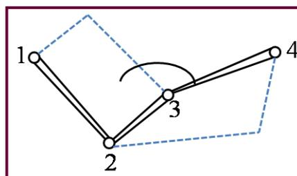
**Figure 2.6 Torsional angle**
