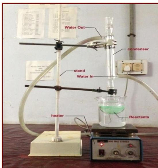
**Figure 2.2** Experimental setup for reflux method
