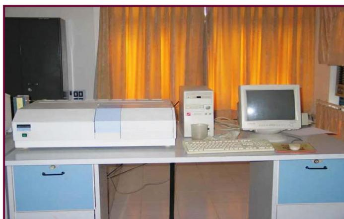
**Figure 2.13** Perkin Elmer Lambda 19 Spectrometer
