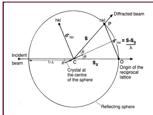
**Figure 2.1 The “Ewald Sphere” construction**
