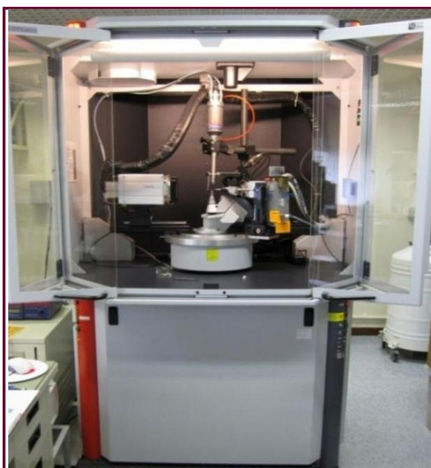
Figure 2.4 Bruker AXS Kappa Apex II CCD 4 diffractometer
