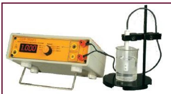
**Figure 2.14** EQ-660 Conductivity meter
