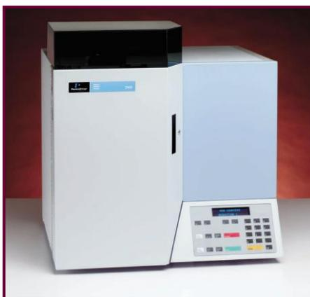
**Figure 2.10** CHN analyzer
