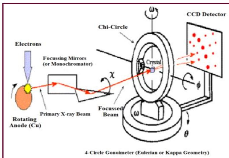
Figure 2.3 Schematic diagram of CCD 4 diffractometer
