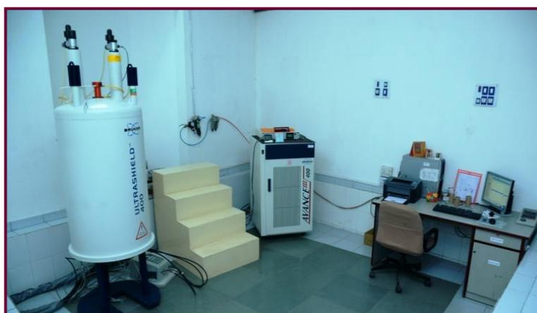
**Figure 2.12** NMR Spectrometer
