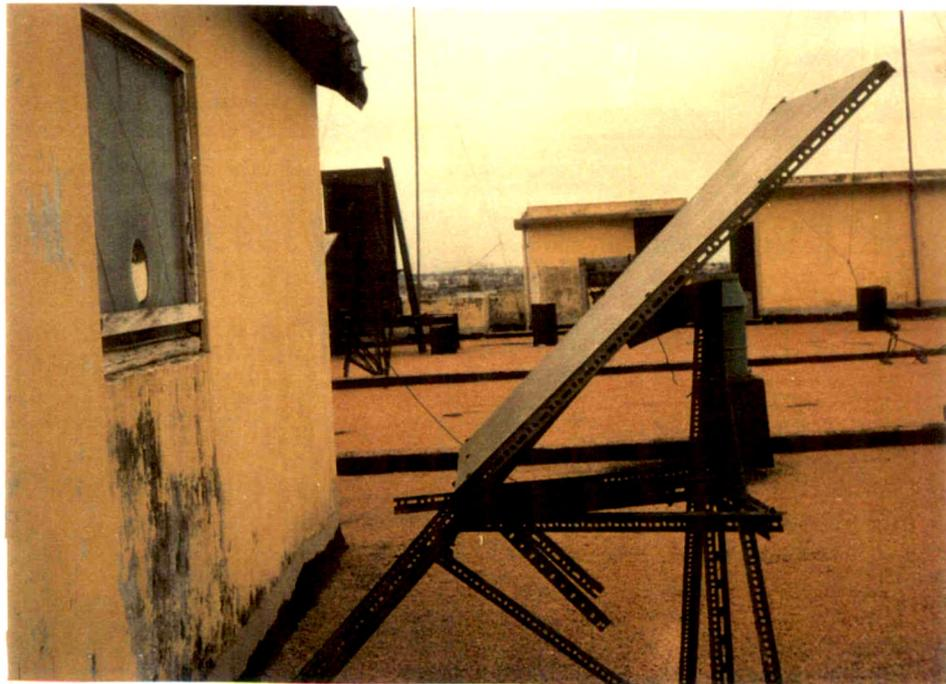
**Fig.2.3** The metallic reflector kept at  $45^\circ$  inclined to the ground outside the room.
