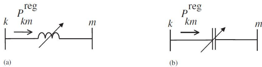
Figure 3.8 Thyrister controlled series compensator equivalent circuit (a) Inductive and (b) capacitive operative region
