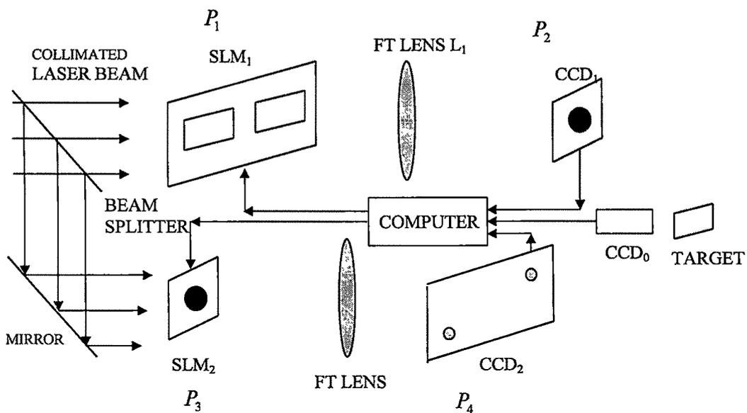
Figure 3.1 Schematic diagram of optoelectronic implementation of JTC
