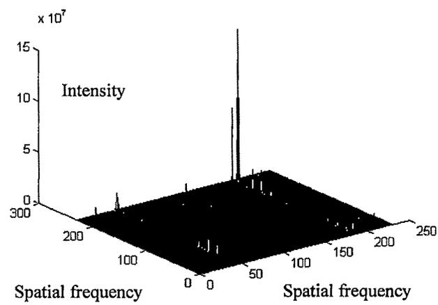
**Figure 3.8d Correlation peaks showing the existence of a thick yarn**
