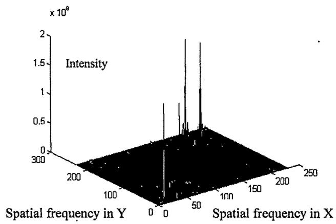
**Figure 3.8b** Correlation peaks showing the presence of two knots and their position in test fabric.
