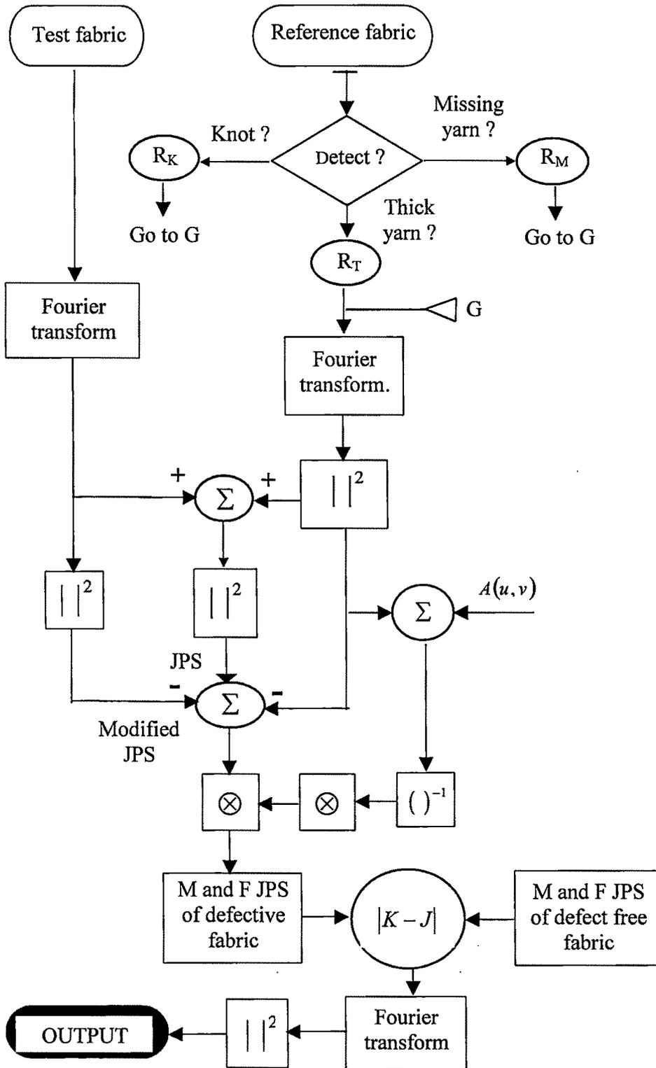
Figure 3.7 Flow chart of the joint transform correlation technique
