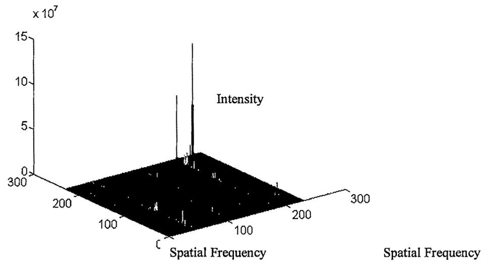
**Fig 3.8c Correlation peaks for identification of missing yarns**
