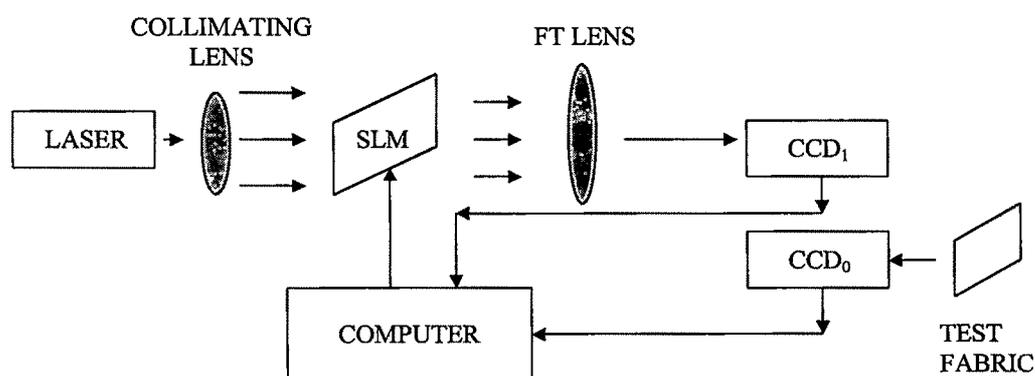
Figure 3.2 Experimental setup for JTC using single SLM
