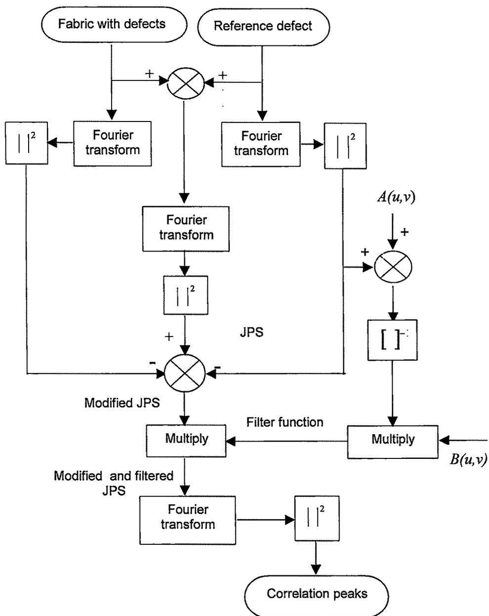
Figure 3.3 Flow chart for joint transform correlation processing
