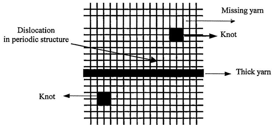
**Figure 3.8a** Constructed test fabric for simulation
